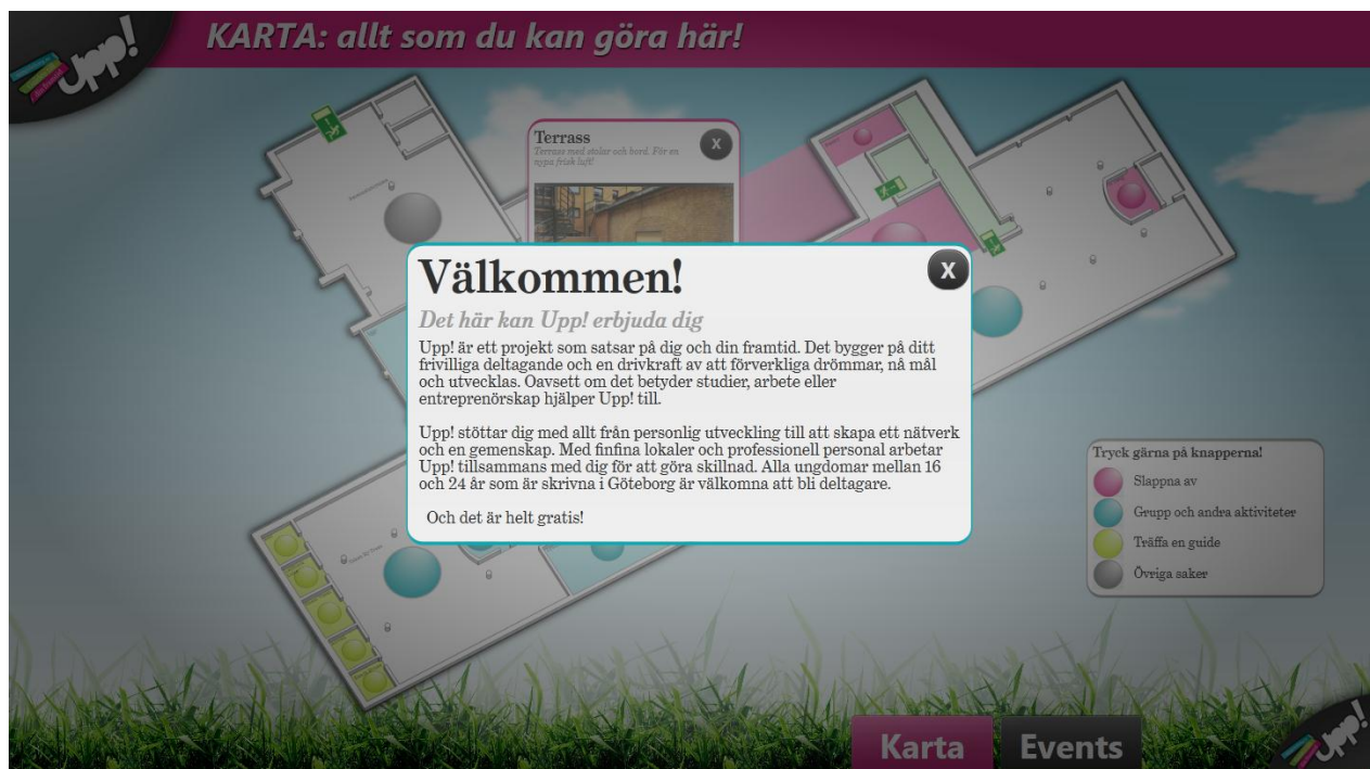
Figure 32: The welcome screen, activated by clicking the Upp logos, top left and bottom right corner in diagonal balance. It closes just by tapping the message, and not only the X, to accommodate short people.
