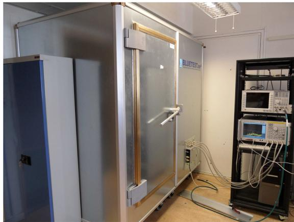
**Figure 3.18:** The BLUETEST reverberation chamber and the Aglient E5071C network analyzer; Chalmers antenna group
