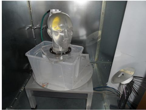
**Figure 3.20:** Efficiency measurement in reverberation chamber
