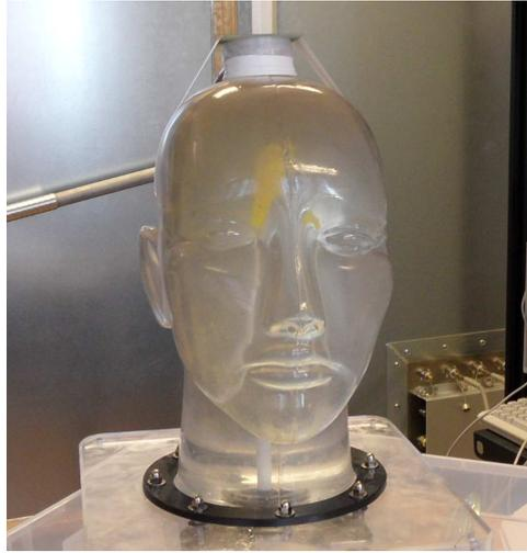
Figure 4.22: The phantom head with one antenna on top to measure S-parameter
