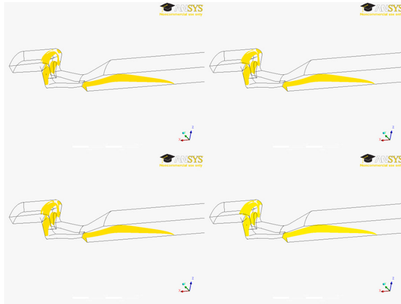
Figure 25. Recirculation zones; Top row: 400K(left) and 500K (right);Bottom row: 1M (left) and 2M (right)
