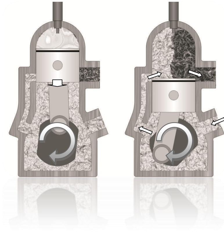
Figure 2-1 The two stroke engine
