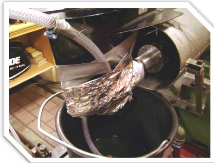
Figure 5-4 Cooling of gearbox
