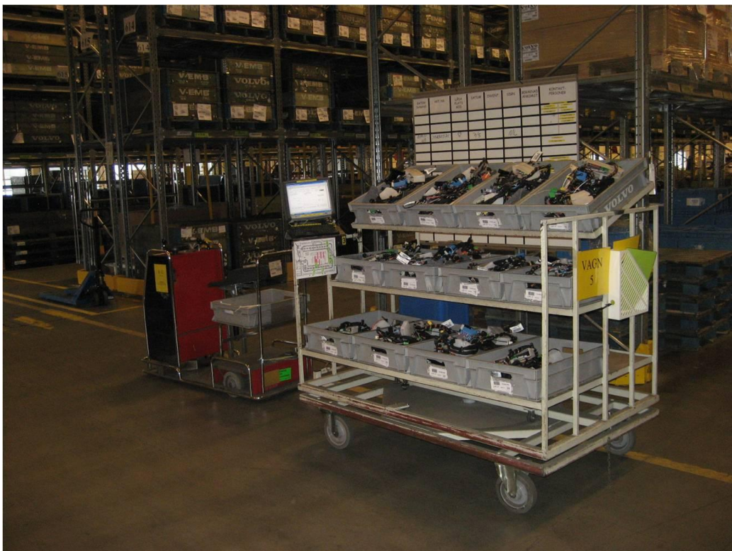
Figure 18. Hand-held truck with attached carriage used in the picking process
