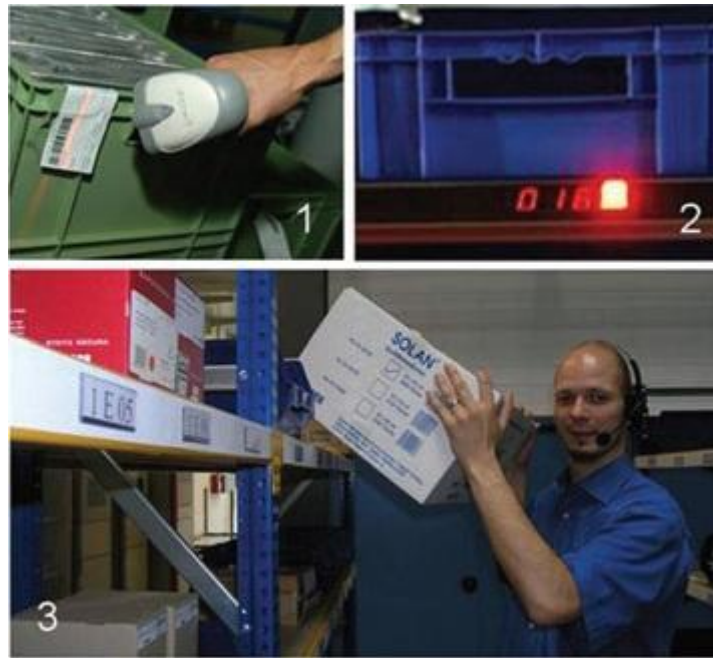
Figure 10. Different picking aids: bar code scanner (1), pick-to-light (2) and pick-to-voice (3) (Reif et al., 2010).
