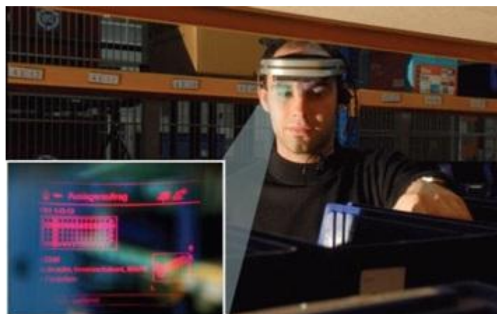
Figure 11. Head-mounted display for visual picking support (Reif et al., 2010).
