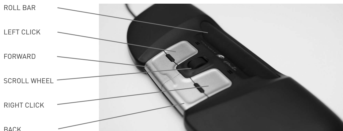
Figure 6.1 The functions of the Trackbar, which caused some confusion for many users.
