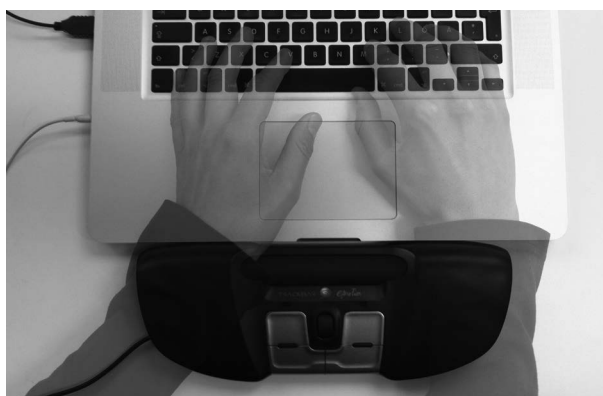
Figure 6.5 Using Trackbar with a laptop causes a lot of reaching.
