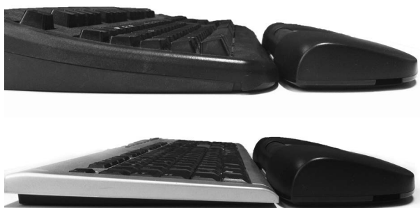
Figure 6.4 Trackbar used with a regular thick keyboard (top) and with a flat keyboard (bottom).
