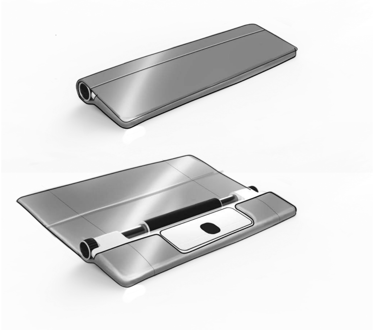
Figure 13.9 A sketch proposal for a sleeve solution, protecting the device during transportation and adding extra features.
