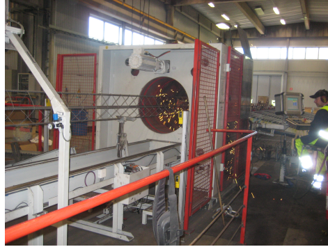
Figure 2.2: Automatic production of reinforcement for concrete foundation piles using resistance welding.
