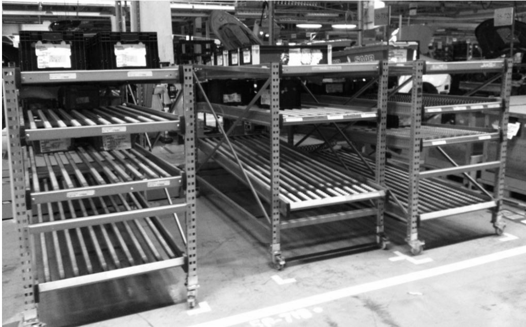
Figure 12: Line side storage rack for Antenna
