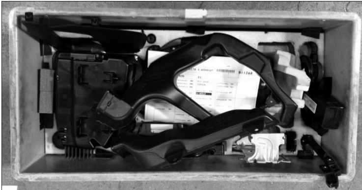
Figure 7: Kit container for Dashboard panel assembly line
