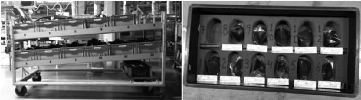
Figure 8: Picture of rack and box for Antenna
