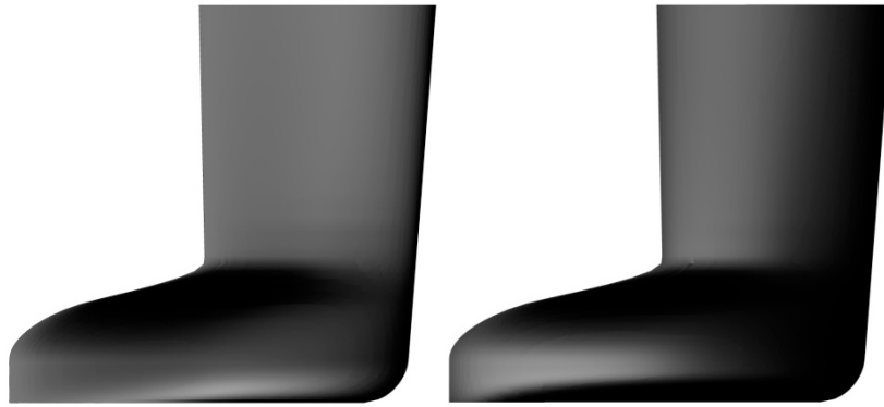
Figure 5.3 Profile view of the initial (left) and optimised (right) keel design
