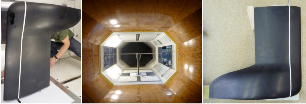
Figure 3.7 The keel mounted in the wind tunnel, the keel model in the wind tunnel, a side view of the keel model.
