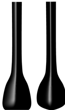
Figure 5.2 Front view of the initial (left) and optimised (right) keel design
