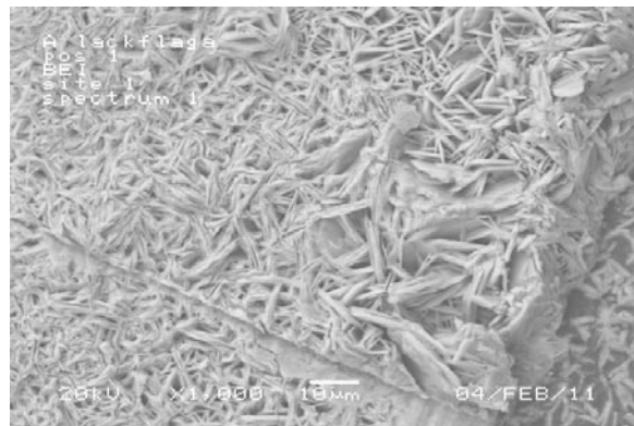
Figure 4.3. SEM picture from backside of paint position A. Needle like crystals are seen.
