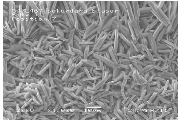
Figure 4.5. SEM picture from backside of paint position C. The crystals are formed as hexagonal plates.
