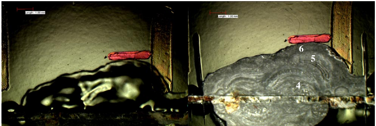
Figure 4.15. Corrosion spreading on material B. The scribe is in both pictures at the bottom of the picture. The left picture is with coating and in the right picture the coating has been peeled off. The markings 4-6 represent analyzing spots.
