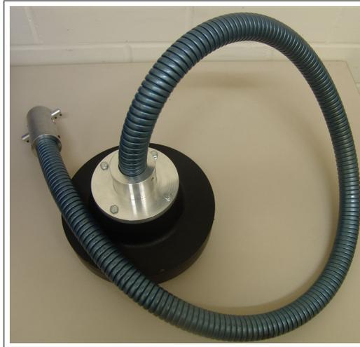
**Figure II-2:** The self constructed volume sound source of the LuK GmbH & Co. KG
