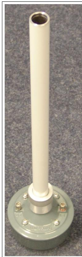
**Figure 3-2:** The self-made volume sound source
