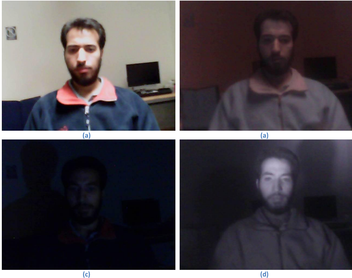
Figure 3.5: Image capture from Visual and NIR webcam: a) Visual Image (Day) b) NIR image (Day) c) Visual Image (Night) d) NIR Image (Night)
