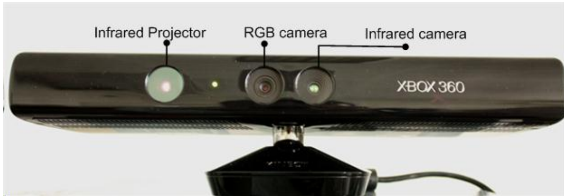
Figure 3.7: Different components in Microsoft Kinect
