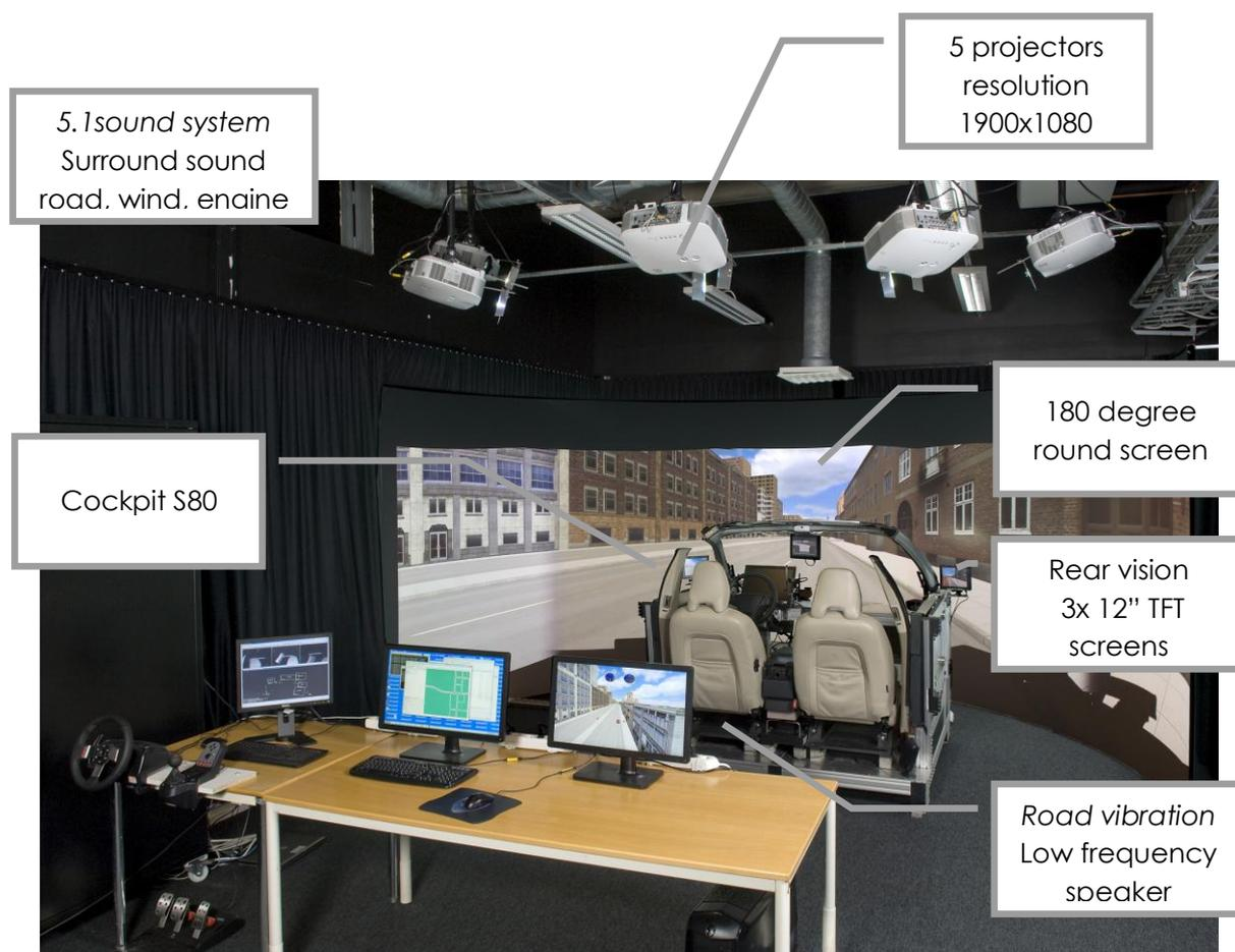
Figure 4.1 Simulator at Volvo HMI laboratory
