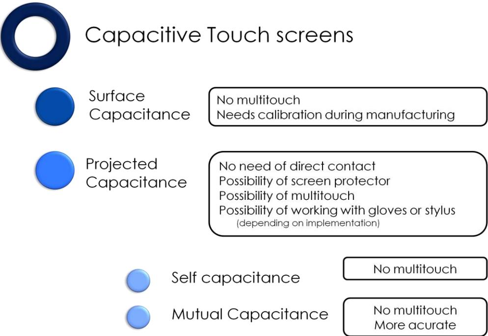
Figure 2.1 Types of capacitive touch screens.
