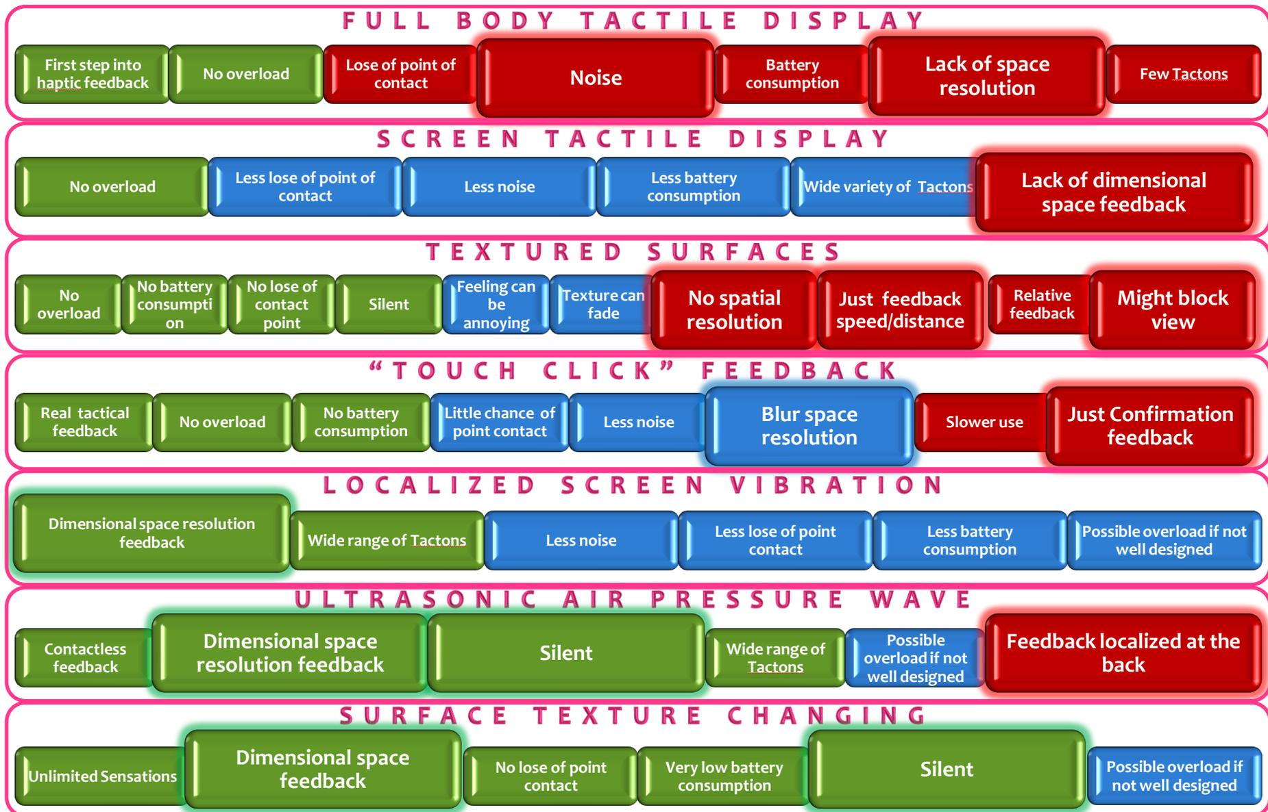
Table 3.3 Comparison between technologies to create haptic feedback on touch screen with highlighted key information
