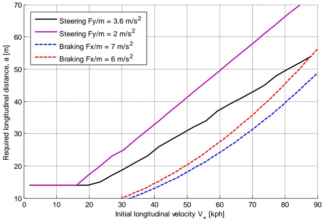
Figure 5.24 Required longitudinal distance versus initial longitudinal velocity.
