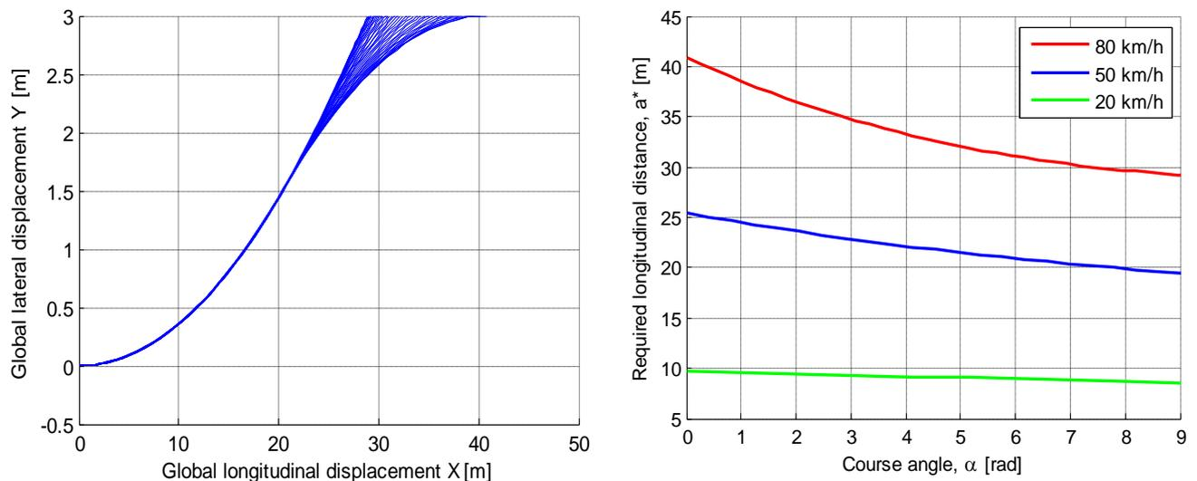
Figure 5.4 Required longitudinal distance versus final course angle.
