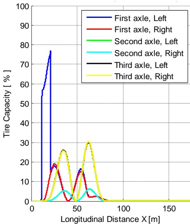
Figure 5.21 Tire force capacity with turn in braking.
