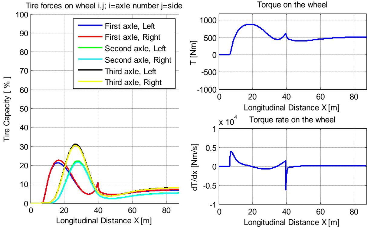
Figure 6.10 Path control results for RORP scenario tire capacity and the torque profile.
