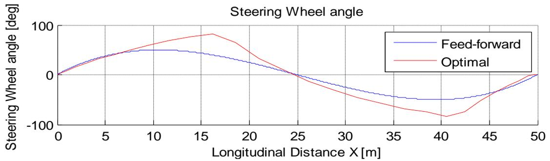
Figure 5.10 Optimal control versus feed-forward steering angle
