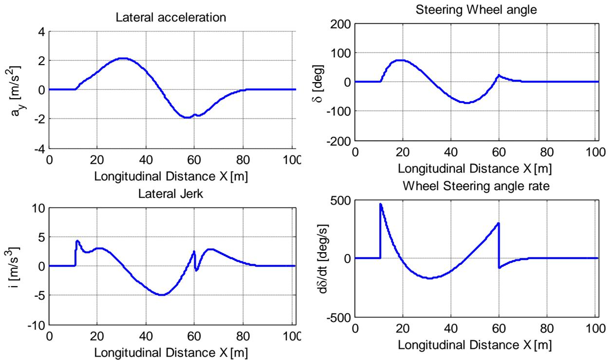
Figure 5.15 Path stability control results for integrated steering-braking actuator configurations for RECA. lateral acceleration, steering wheel angle and the torque and steering angle rate.
