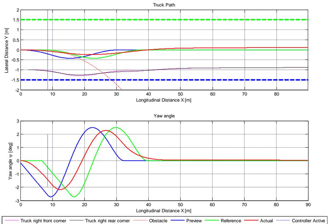
Figure 6.3 Path stability control results for RORP scenario- position and heading angle
