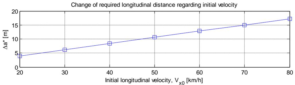
Figure 5.3 The amount of change in longitudinal distance ( $\Delta a^*$ ) by reducing the lateral distance  $b$  from 3 to 1.
