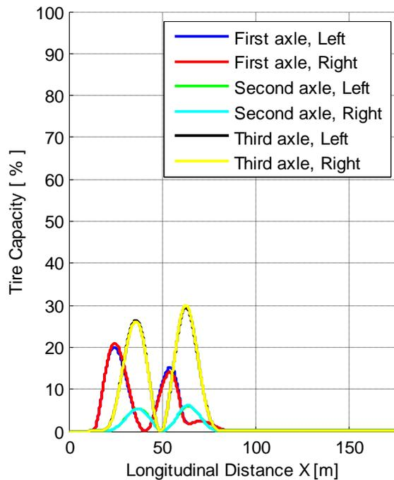
Figure 5.18 Tire force capacity without turn in braking.
