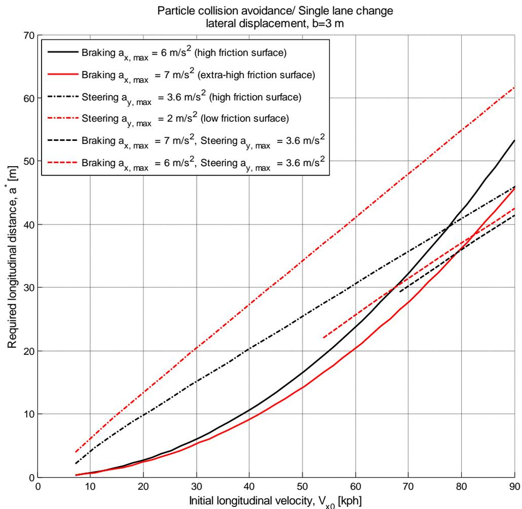
Figure 5.1 Required longitudinal distance versus initial longitudinal velocity.
