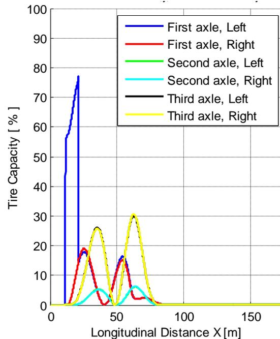
Figure 5.19 Tire force capacity with turn in braking.
