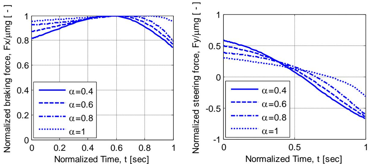
Figure 5.6 Steering-braking integration regarding the maneuver severity
