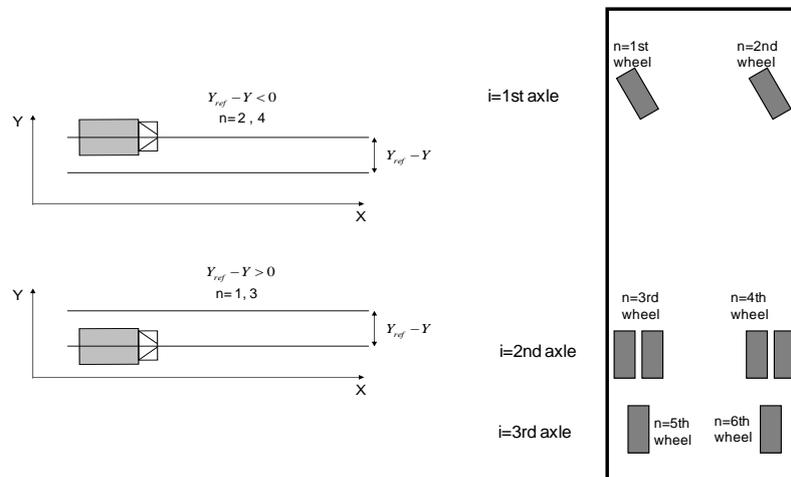
Figure 4.4 Schematic sketch of the braking stability control.
