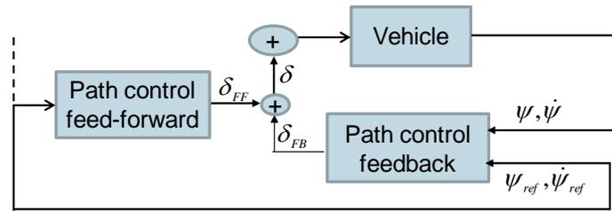
Figure 4.3 Schematic sketch of path stability controller.
