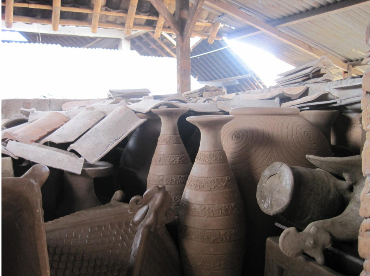
Figure 3 A densely packed furnace covered with a layer of tile but no straw. Everything is packed randomly and small items are placed between bigger ones.
