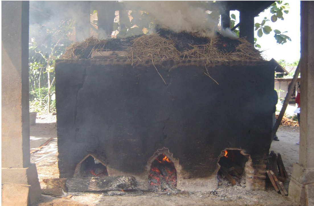
Figure 1 Traditional updraft pottery furnace
