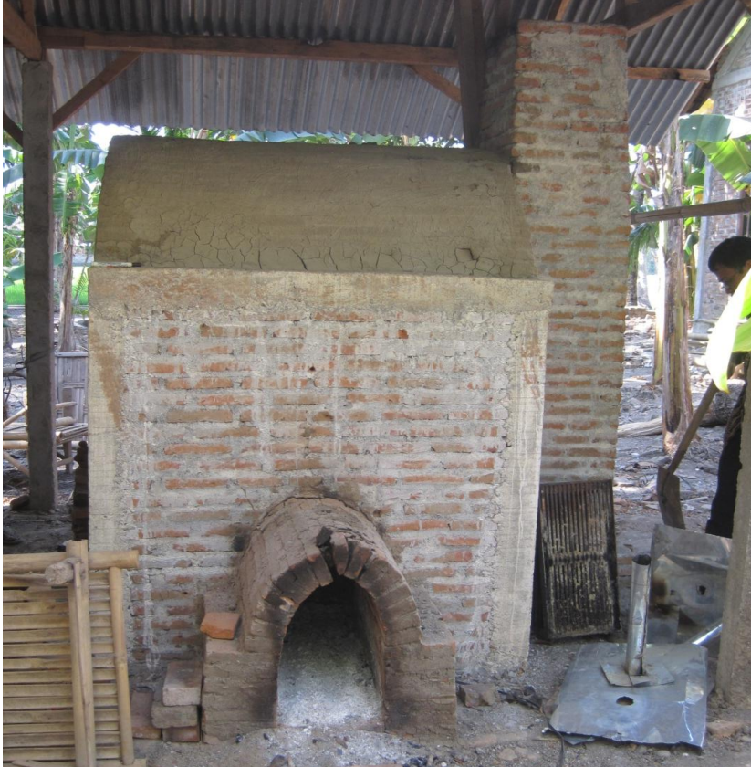
Figure 2 A slightly more modern version of a traditional pottery furnace that has downdraft.
