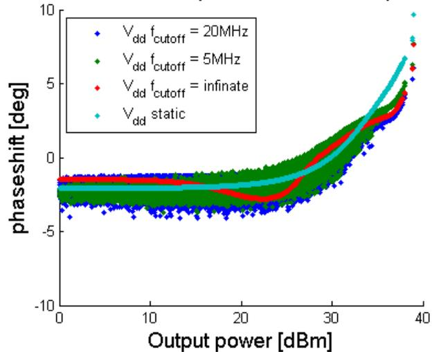
Figure 23. Predicted AM/PM behaviour when employing DSM.
