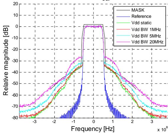
Figure 24. MATLAB simulation comparing desired output signal with simulated response for an output power of 30dBm.
