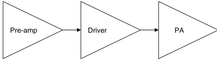
**Figure 32. Transmitter amplifier stages.**
