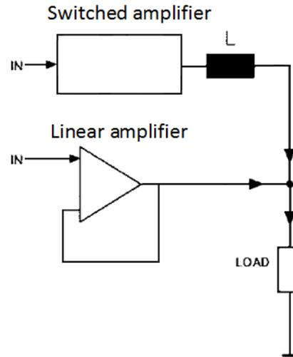
**Figure 33. Conceptual description of the Envelope amplifier.**
