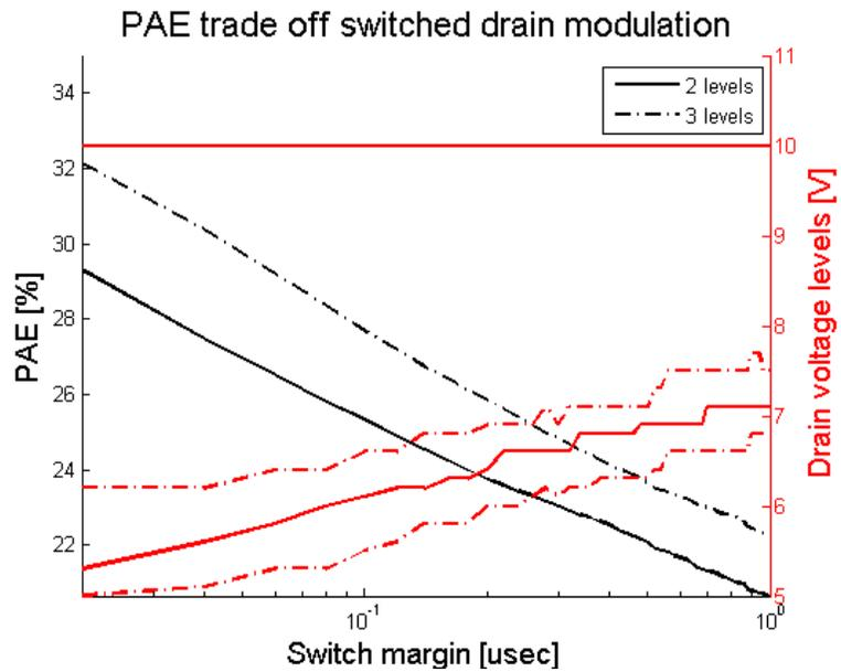
**Figure 19. PAE improvement potential estimation for switched drain modulation. The term switch margin refers to the time between when a switched is set on and the value is reached.**
