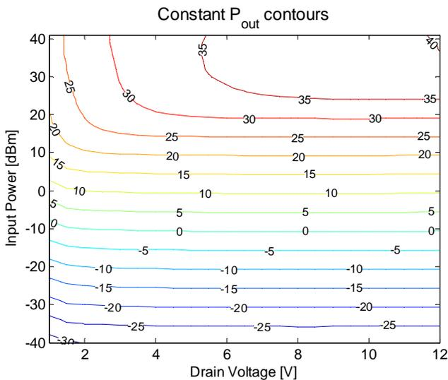
Figure 15. Constant  $P_{out}$  contours produced using the data from the PA characterization.
