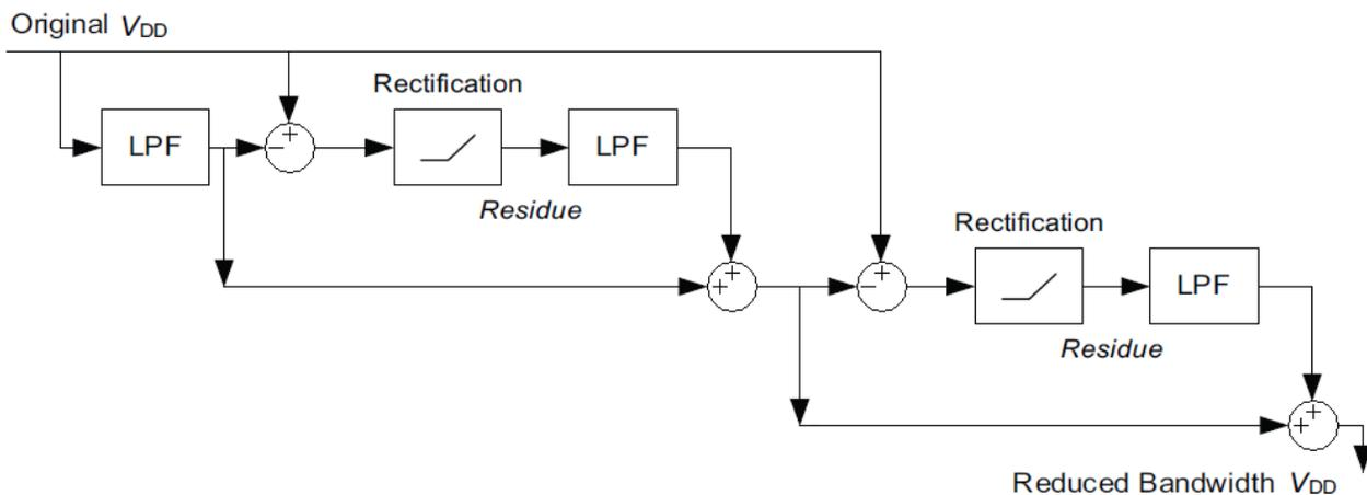
**Figure 20. Schematic description of the iterative peak tracking low pass filter.**
