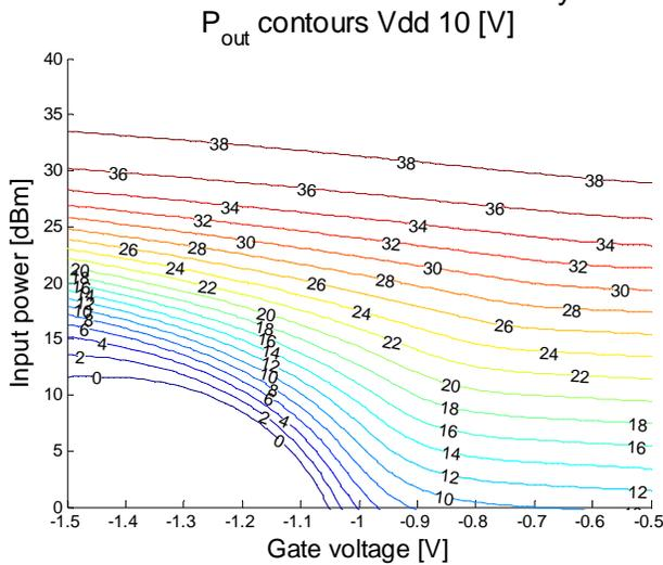
Figure 9.  $P_{out}$  as a function of  $V_{gs}$  and  $P_{in}$  simulated with  $V_{dd} = 10V$ .
