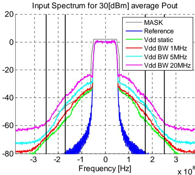
Figure 26. Spectral growth of input spectrum with DSM for 30dBm average Pout.
