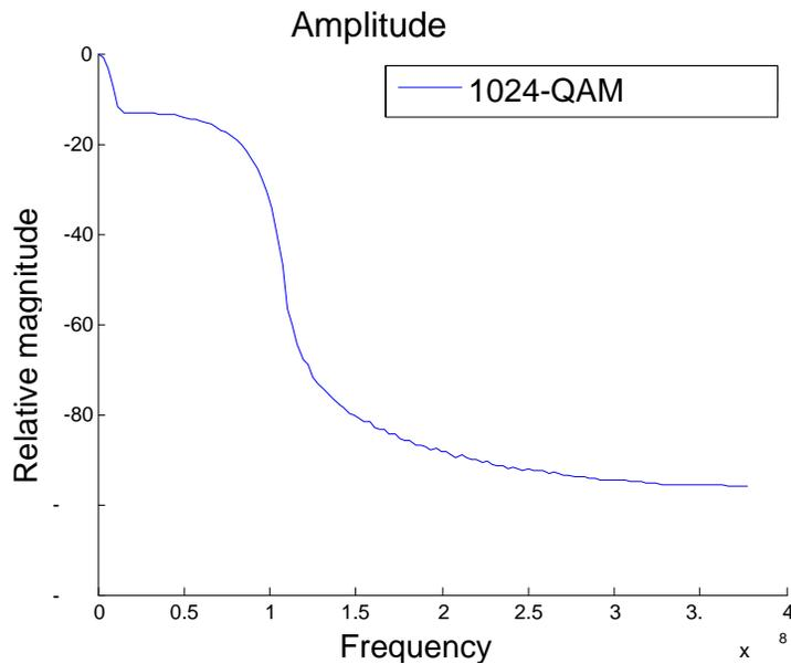
**Figure 4. QAM-1024 envelope bandwidth.**
