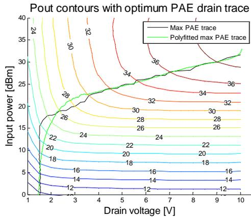
Figure 11. Optimum PAE trajectory and polynomial fit on top of with constant P<sub>0</sub>out contours.
