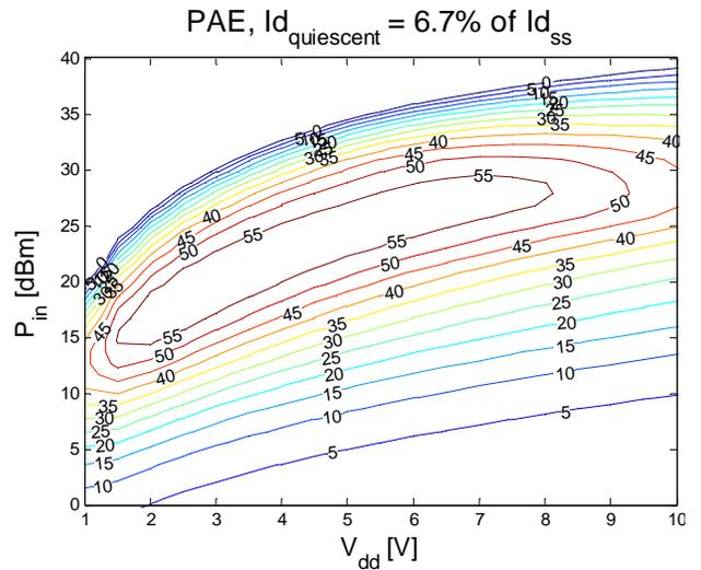
Figure 8. PAE as a function of  $V_{dd}$  and  $P_{in}$  simulated with  $I_{d_{quiescent}} = 6.7\%$  of  $I_{d_{ss}}$ .
