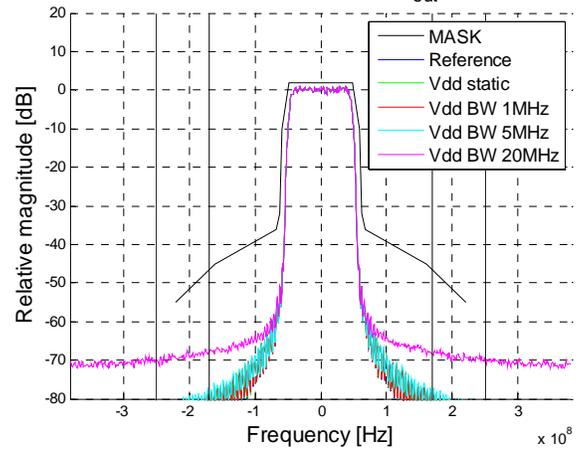
Figure 25. MATLAB simulation comparing desired output signal with simulated predistorted response for an output power of 30dBm.
