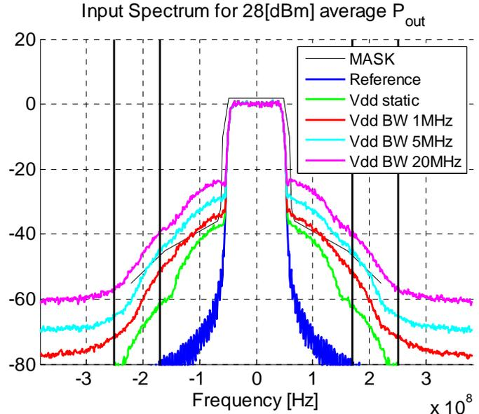
Figure 27. Spectral growth of input spectrum with DSM for 28dBm average Pout.
