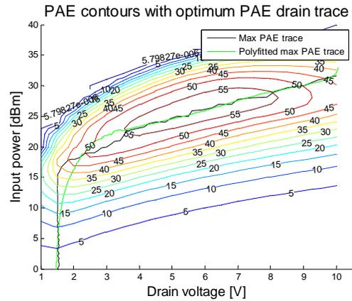
Figure 13. Optimum PAE trajectory and polynomial fit on top of constant PAE contours.
