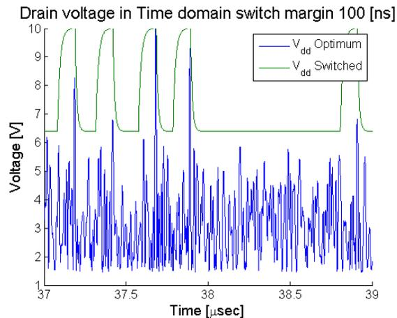
**Figure 3. Example of drain voltage signal comparing optimum dynamic drain bias modulation and a switched taking rise and fall time into account.**
