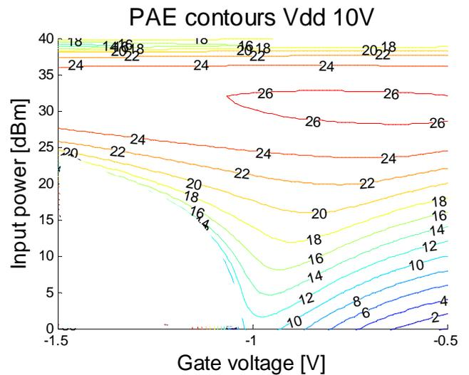
Figure 10. PAE as a function of  $V_{gs}$  and  $P_{in}$ .
