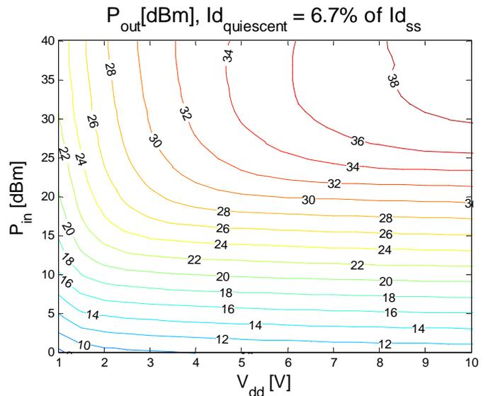
Figure 6.  $P_{out}$  as a function of  $V_{dd}$  and  $P_{in}$  simulated with  $I_{d_{quiescent}} = 6.7\%$  of  $I_{d_{ss}}$ .
