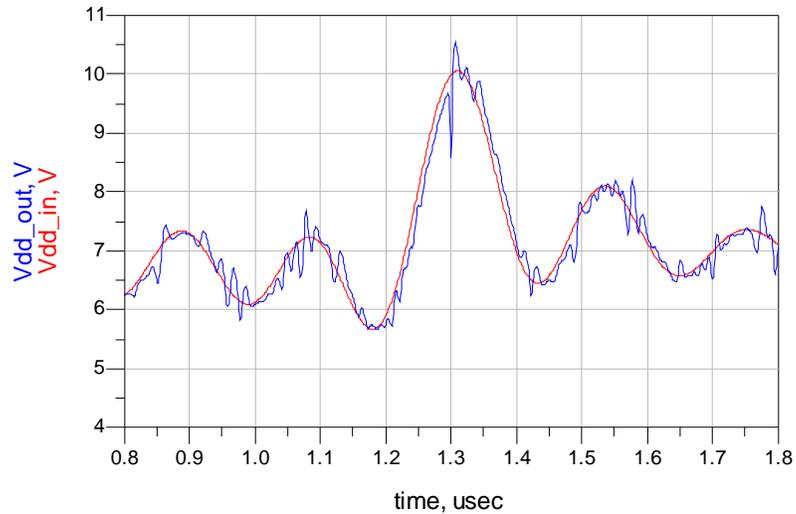
**Figure 38. Comparison of input and output signal of the linear amplifier for a QAM-1024 modulated drain voltage signal bandwidth reduced to 5 GHz simulated with an ADS model PA as load.**
