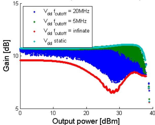
Figure 22. Predicted AM/AM behaviour when employing DSM.
