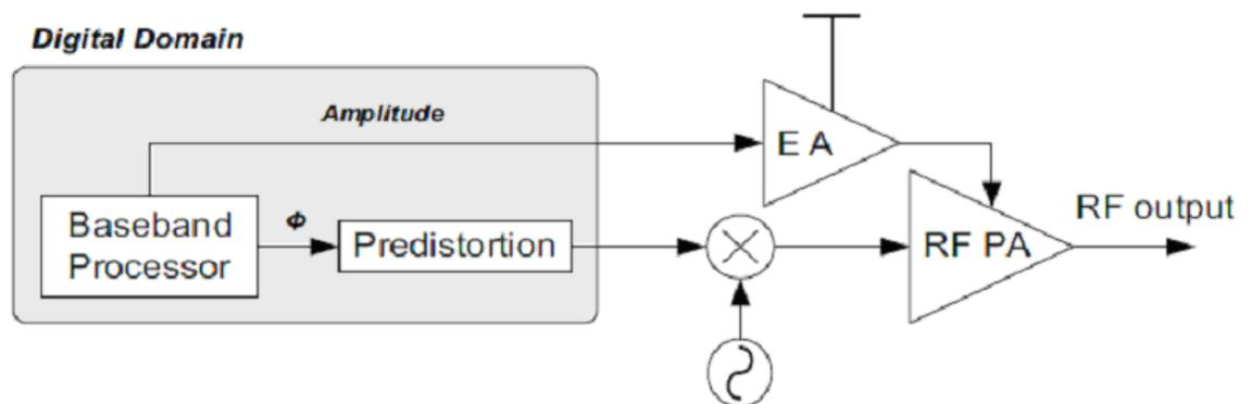
Figure 2. Basic concept of digitally controlled Envelope tracking.
