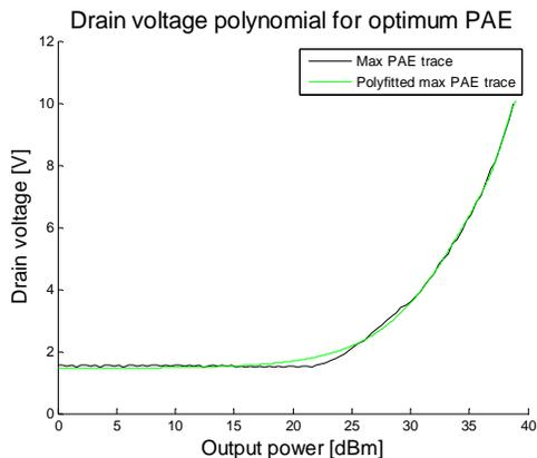
Figure 12. Example of drain voltage polynomial fitted onto the optimum trajectory.
