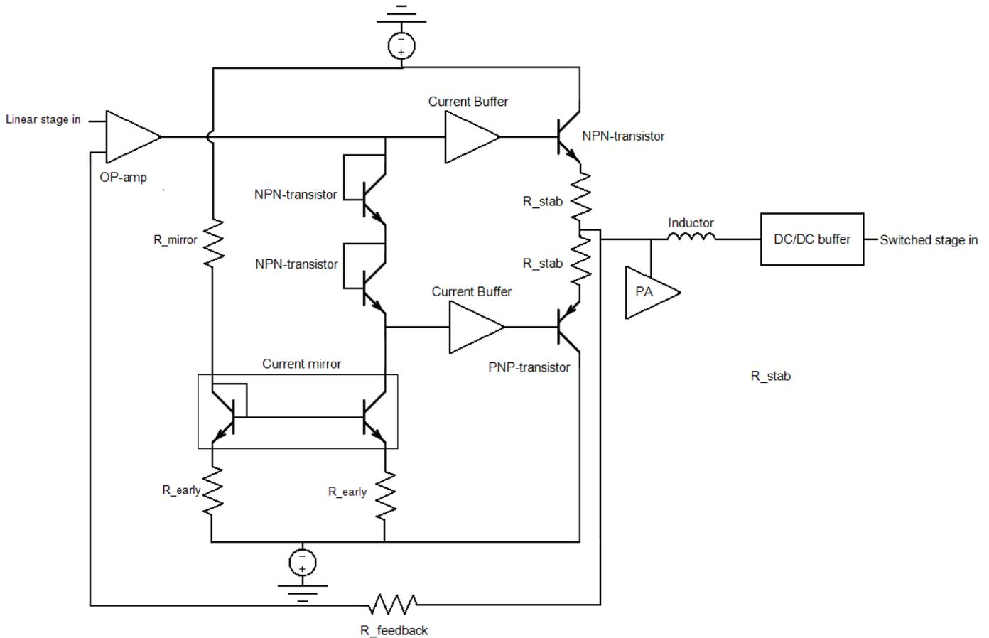
**Figure 35. Envelope amplifier conceptual layout.**
