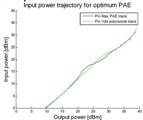
Figure 14. Example of Pin trajectory calculated from the V<sub>dd</sub> polynomial.
