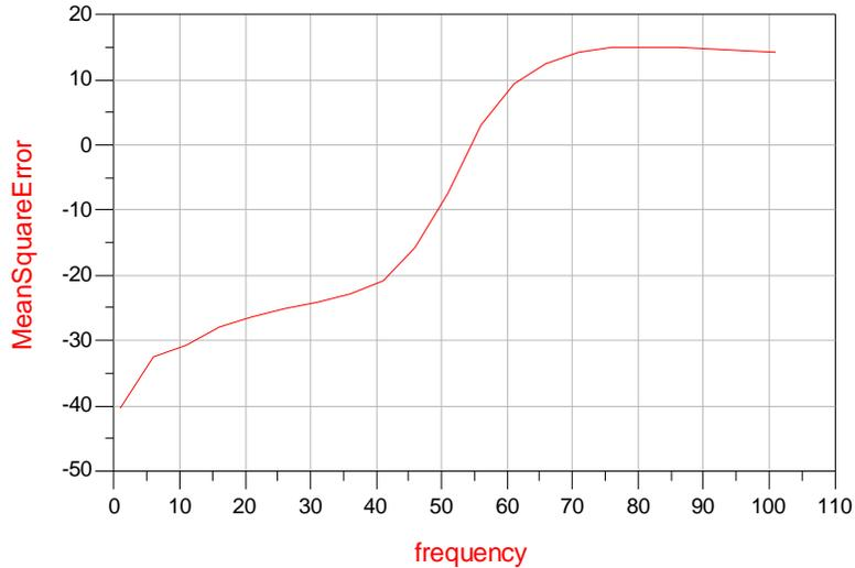
**Figure 36. Linear Envelope amplifier MSE as a function of frequency.**
