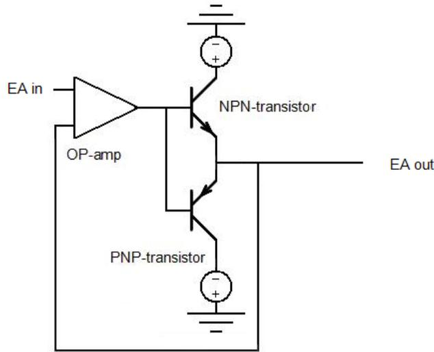
**Figure 34. Basic push pull feedback loop.**
