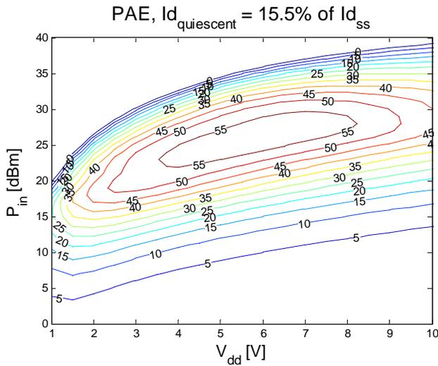
Figure 7. PAE as a function of  $V_{dd}$  and  $P_{in}$  simulated with  $I_{d_{quiescent}} = 15.5\%$  of  $I_{d_{ss}}$ .
