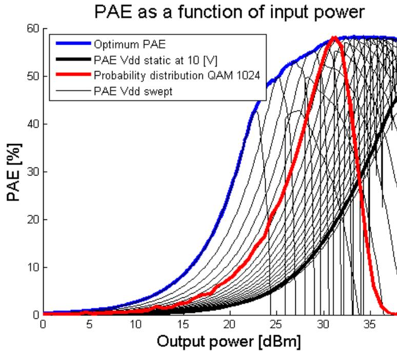
**Figure 17. PAE as a function of output power for various drain voltage supply levels. Comparing the dynamic range for drain modulation with the probability distribution of a 1024-QAM signal. Vdd range from 1V to 12V, with gate bias set to 15.5% of  $I_{d_{ss}}$ .**
