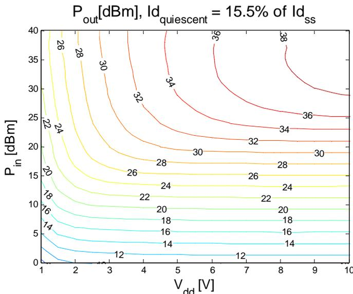
Figure 5.  $P_{out}$  as a function of  $V_{dd}$  and  $P_{in}$  simulated with  $I_{d_{quiescent}} = 15.5\%$  of  $I_{d_{ss}}$ .
