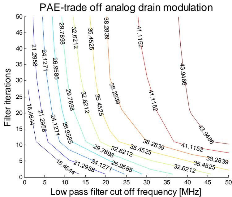
Figure 21. Trade off between LPF cut off frequency and number of filter iterations for bandwidth reduced dynamic drain modulation.
