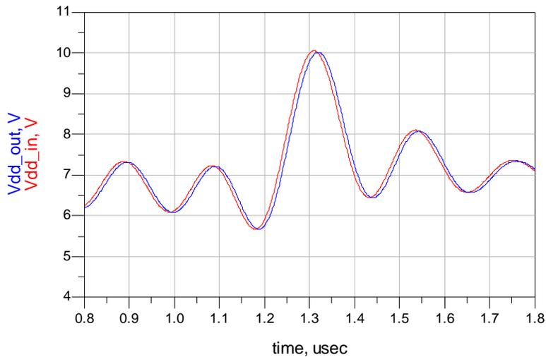
**Figure 37. Comparison of input and output signal of the linear amplifier for a QAM-1024 modulated drain voltage signal bandwidth reduced to 5 GHz simulated with a resistive load.**
