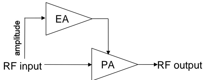
Figure 1. Envelope tracking architecture.
