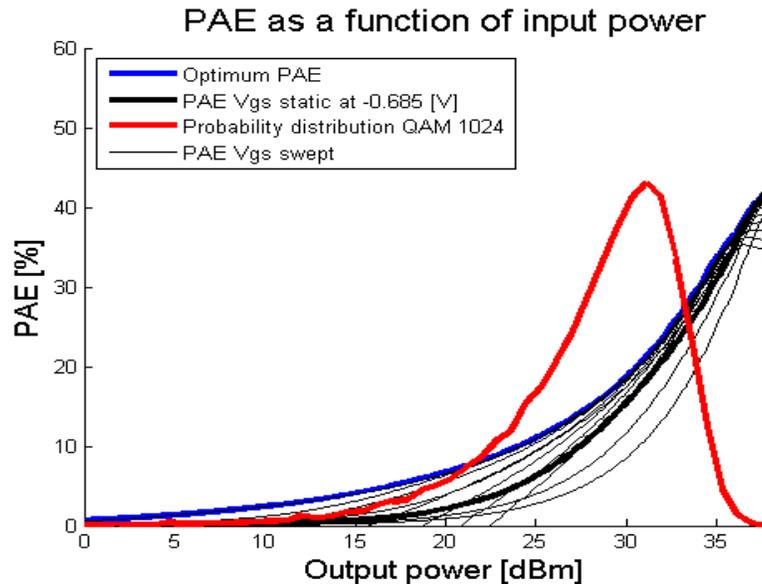
Figure 18. PAE as a function of output power for various gate voltage supply levels. Comparing the dynamic range of gate modulation with the probability distribution of a 1024-QAM signal.  $V_{gs}$  from -1.5V to -0.5V.
