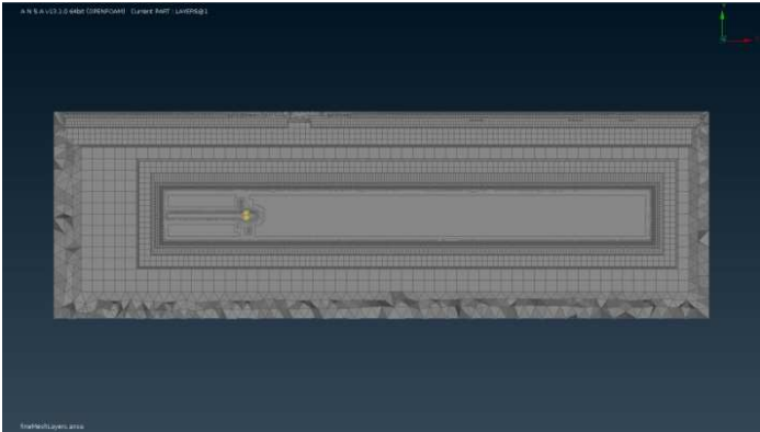
Fig. 8.12: The fine mesh used for the velocity field measurement
