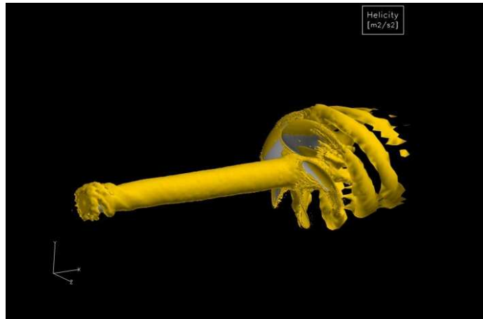
Fig. 8.13: Tip vortex with helicity of 150 \text{ m}^2/\text{s}^2 at the working point
