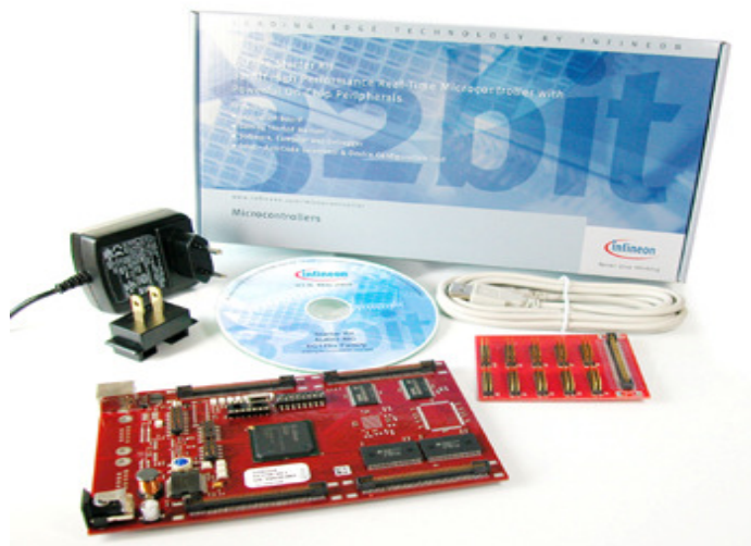
Figure 6 - TriBoard TC1797 from Infineon
