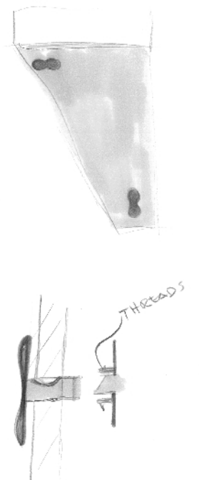
Figure 9-9 Another attachment principle, where the package is attached by rotating a handle 90 degrees, screw to fasten.
