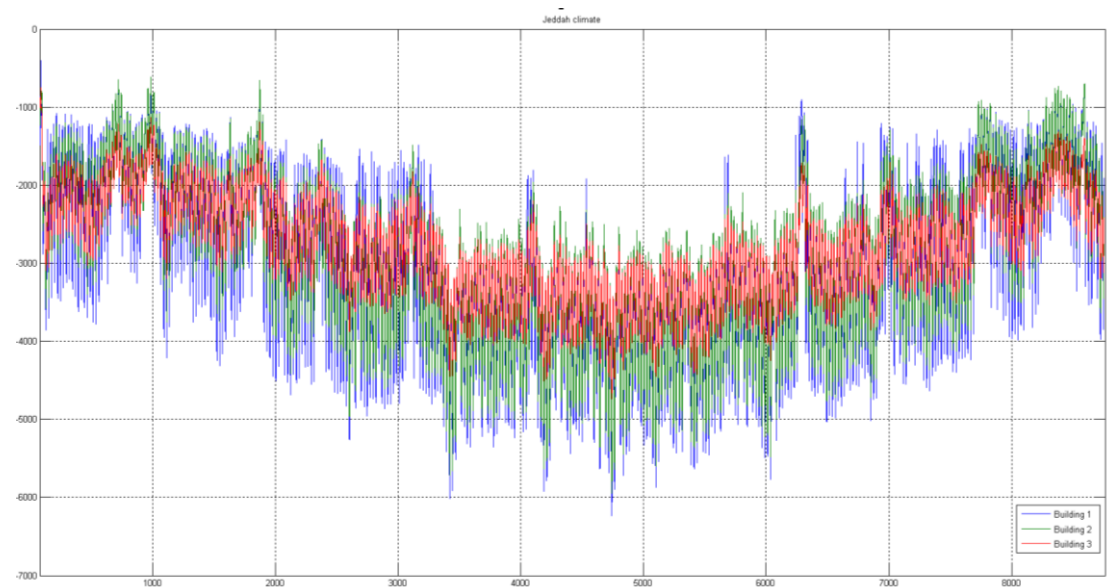
Figure 29 Fan coil cooling load (-7000 to 0W), in Jeddah, for one year (8760h). Building 1 in blue, building 2 in green, building 3 in red. (simulation using the modelling tool Simulink)
