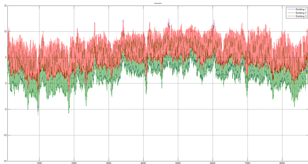
Figure 19 Transmission heat gains through the walls for the different buildings (-15 to 15W/m 2 ) in Jeddah for one year (8760h) [W/m 2 floor area]. (simulation using the modelling tool Simulink)
