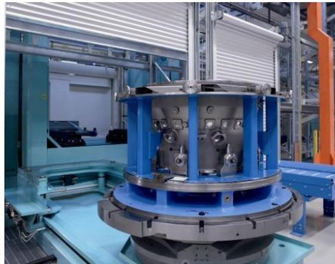
Figure 5: A part mounted into a fixture at a set-up station in the multitask cell.
