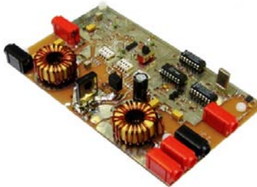
Fig. 3.9: Synchronous step-down converter.
