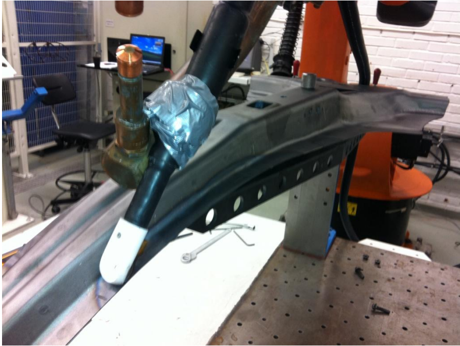
Figure 7: Induction heating of a B-pillar with an industrial robot programmed to move along the flange.
