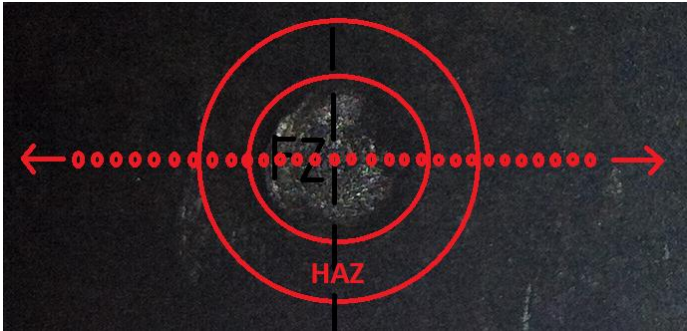
Figure 21: Hardness measured around a spot weld over the cross section of a flange of a tempered B-pillar. The tempering creates a larger soft zone compared to fully hardened B-pillars.
