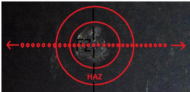
Figure 13: Hardness around spot weld in tempered 22MnB5. Measured over the cross section of a specimen with a weld applied in the middle. The tempering creates a larger soft zone compared to the reference specimen, see Figure 4.
