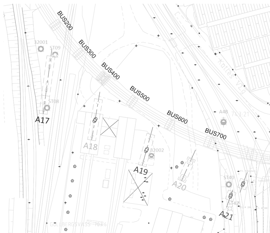
Figure 3.1 Plan drawing; the bridge Skäran, supports A17-A21 for Partihallsbron and seven of the boreholes for the soil investigation.
