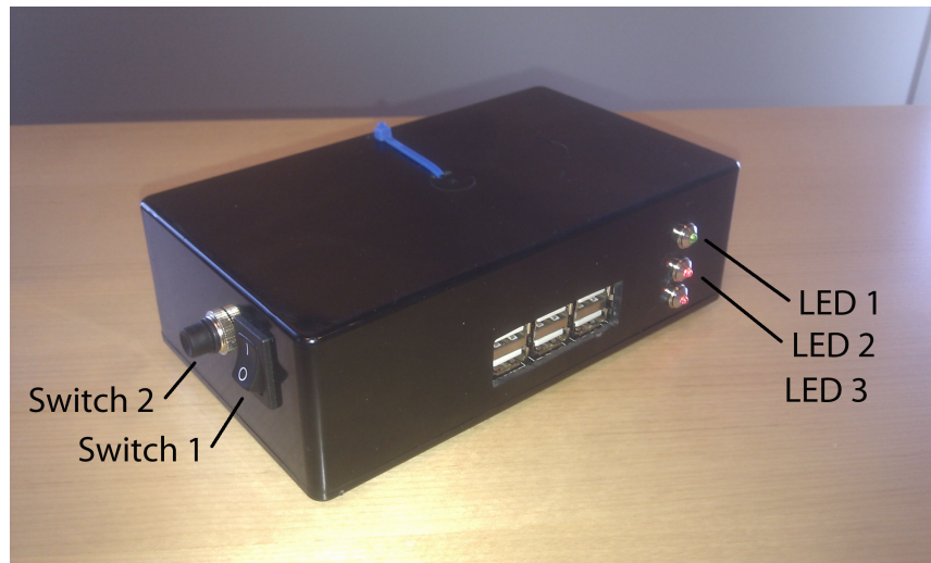
Figure 3.8: The main unit and its casing. Switch 1 is a power switch and switch 2 is used for start and stop logging. LEDs 1-3 are used for giving the user feedback
