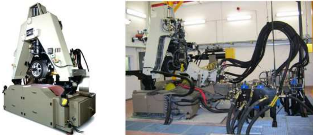
Figure 12: MTS Flat-Trac at the Renault test center of Aubevoye
