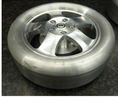
Figure 3.3: The aluminum wheel for the scale model.
