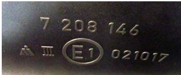
Figure B.1: The E-mark on a left mirror on a BMW 3-serie.
