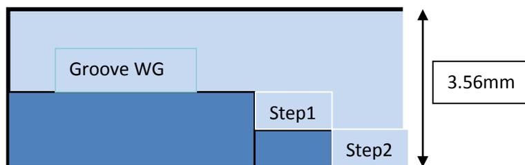
Figure 5-4 Groove gap waveguide with Height adjustments Steps
