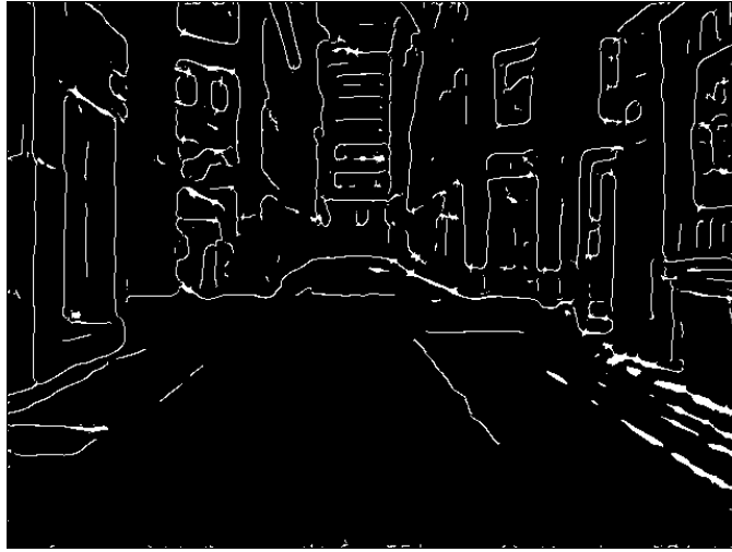
Figure 3.5: Edges detected by implemented Canny edge detector.
