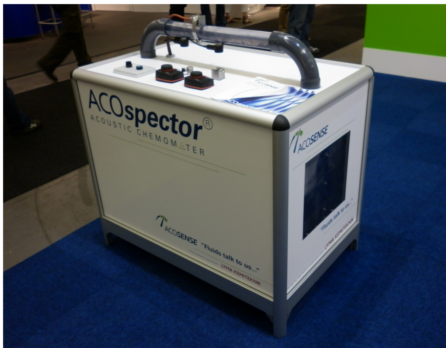
Figure 7.3: The final rig at the SPCI fair in May 2011. On its short side is the window to the water and particles tank. On the top of the rig are the measuring tube with the sound emitter and accelerometers. The black boxes in front of the tube are the controls for flow rate and particle concentration. To the left of them are the button for air bubbles and a power switch.
