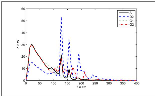
Figure 6. Comparison of dissipated power in the frequency domain for cases A, D2 (lower damping), G1 (higher mass) and G2 (lower mass).
