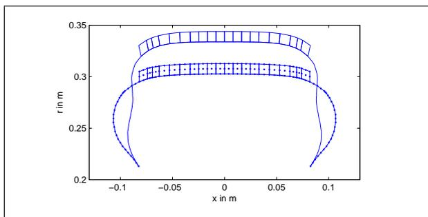
Figure 4. Cross-sectional mode shape for waves of type 127 Hz/order 3 and 156 Hz/order 4. Note: Shown mesh is not the one used in this study.
