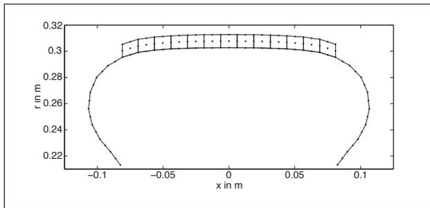
Figure 1. Mesh of the modelled 205/55R16 tyre.
