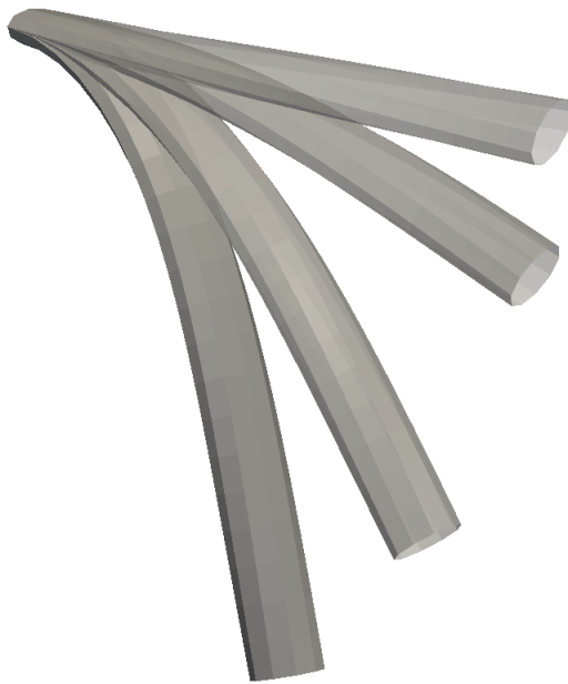
Figure 3.23: Deformed shapes of cantilever beam with twisted elliptical cross section.
