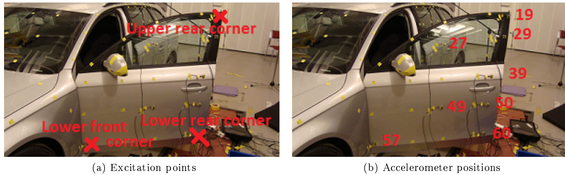
Fig. 5.5: Mobility measurements of the car door of the Audi to find the resonance frequencies.
