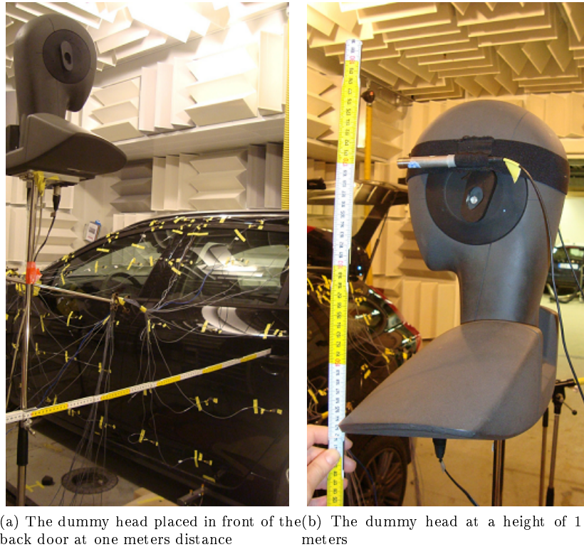
Fig. 4.3: Dummy head set-up
