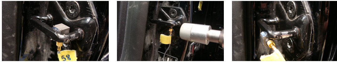
(a) An accelerometer attached in x-direction (b) An accelerometer attached in y-direction (c) An accelerometer attached in z-direction
