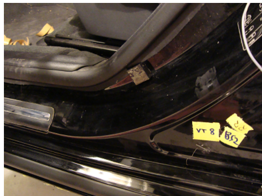
(d) Bump stop in lower corner to increase the damping and facilitate the energy transfer into the car body
