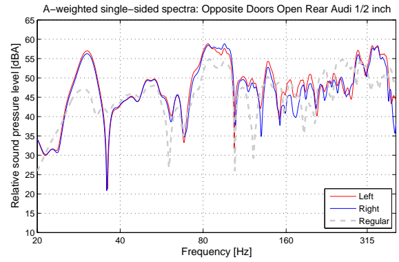
(b) Measurements done while having the opposite doors open for Audi
