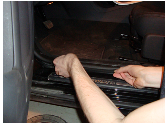
(b) Damping material added to the lower sealing
