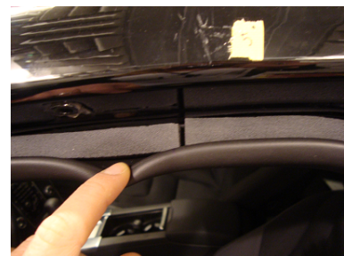
(g) How damping material is positioned under sealing
