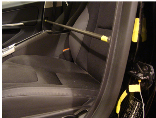
(c) Rod clamped between both B-pillars
