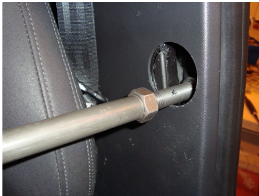
(a) Rod attached to driver's side B-pillar
