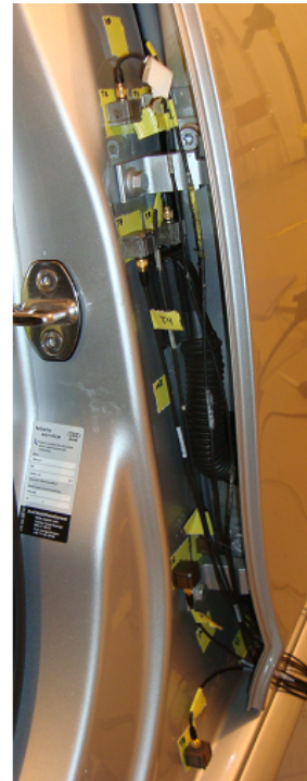
(b) Accelerometers on Audi B-pillar (same numbers as for Volvo)
