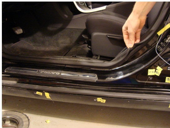
(c) How damping material is positioned under sealing
