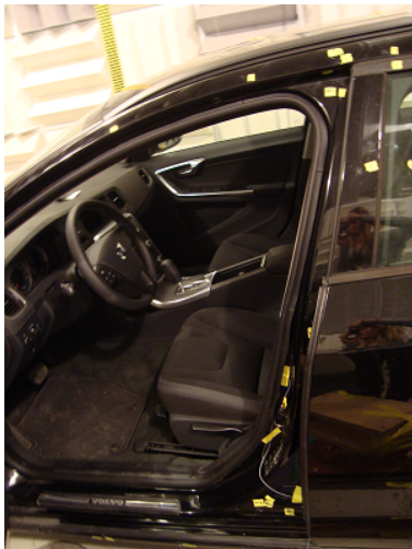
(e) Damping material added to rear seal-
