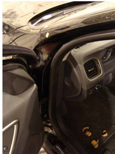
(f) Damping material added to front seal-
