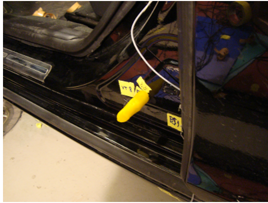
(a) Clay attached to car while closing to find the thickness of the bump stop needed
