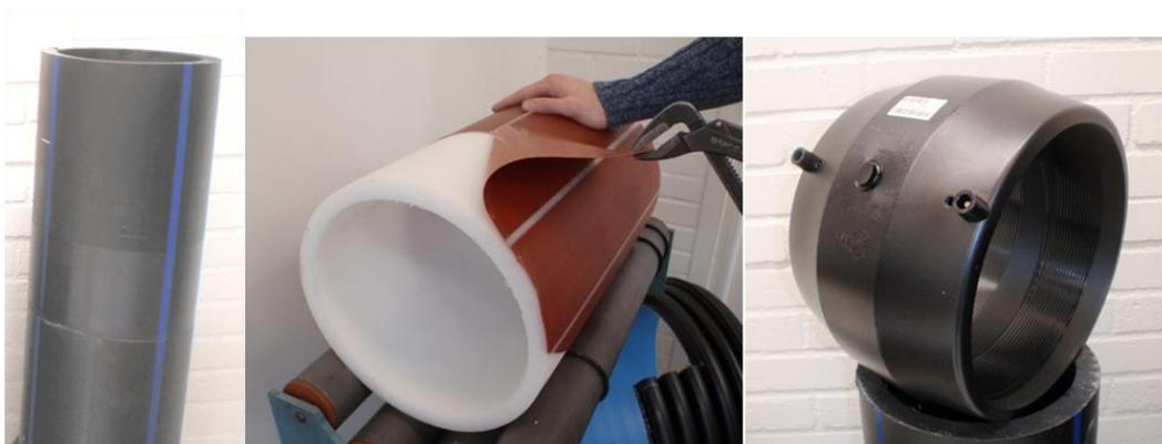
**Figure 10. Materials used for electrofusion welding. Wavin pipe (left), jacketed Profuse pipe (middle) and electrofusion coupler (right).**
