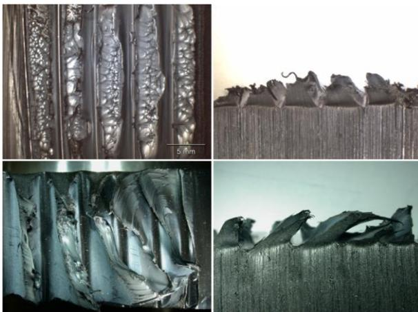
**Figure 7. Typical ductile failures from peel decohesion test showing plastic deformation. Top view to the left and side view to the right.**
