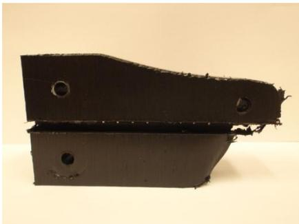
Figure 14. Test sample for double decohesion test with side grooves, which have previously failed in the pipe in peel decohesion test.
