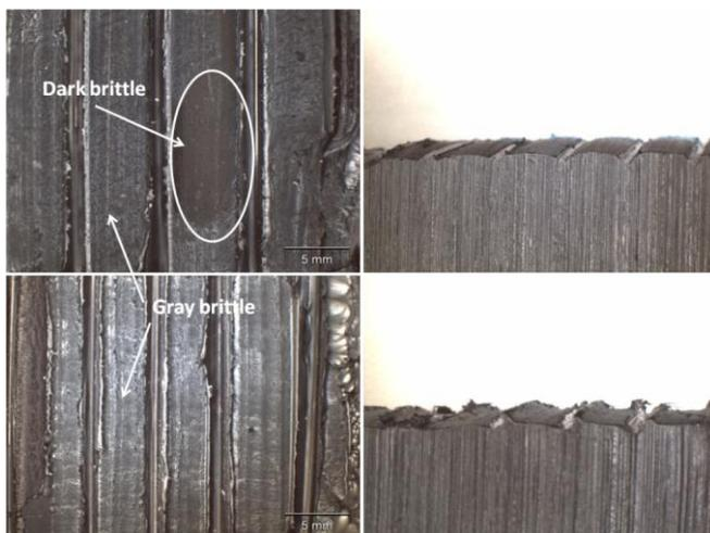
**Figure 9. Typical brittle failures from peel decohesion tests. Notice the different surface appearance, dark black and gray.**
