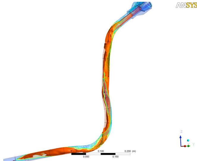
Figure 48. Isosurface plot of the volume fraction gasoline at the walls of the filling pipe for fine prism 17 layers mesh with second order upwind. Simulation time is 0.5s
