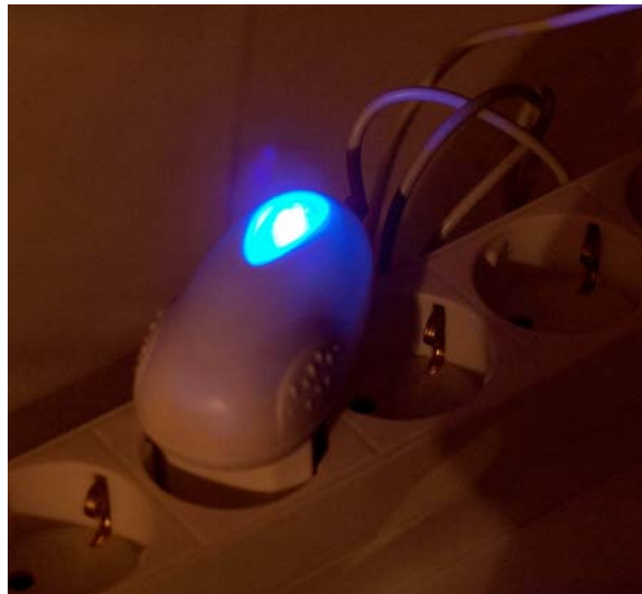
Figure 30. An example of Incentives : a cell phone charger that emits a strong blue light when attached to the socket. If placed in a bedroom, the light may disturb the sleep.
