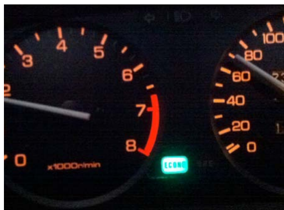
Figure 24. An example of Simple Feedback : in this Honda Civic a green light turns on when you are driving in a fuel-efficient manner.
