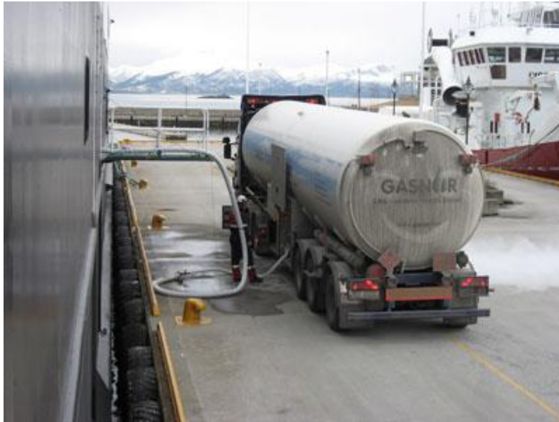
Figure 22 Bunkering procedure between a LNG semitrailer and a receiving vessel (27).
