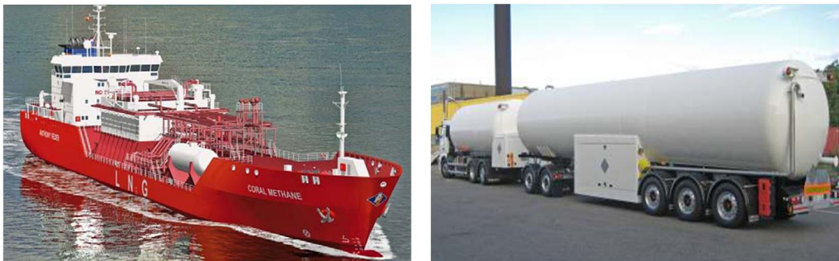
Figure 6 LNG tanker for small-scale marine shipping (7500 m 3 ) (left) (8) and LNG tank truck (80 m 3 ) (right) (11).
