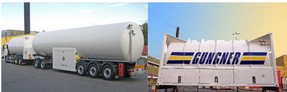
Figure 17 An 80 m 3 Road-trailer (left) and a Cryogenic container (right) (27).
