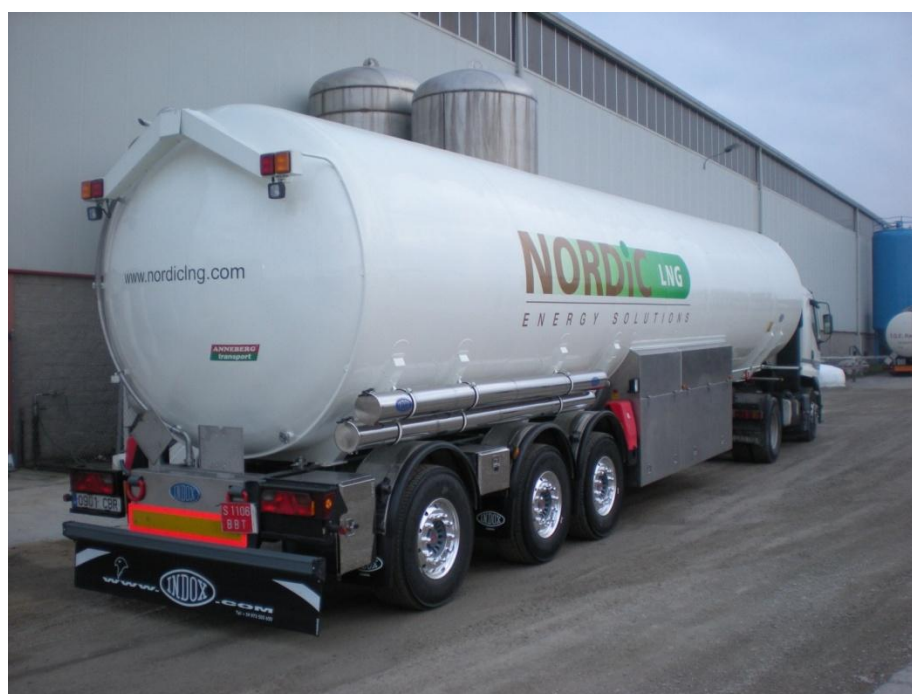
Figure 29 LNG tank truck with a capacity of 50m 3 (33).
