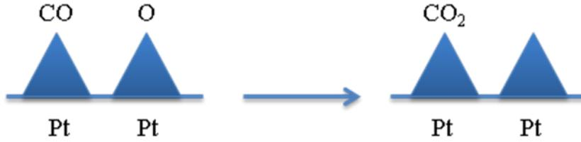
**Figure 4.** A schematic figure of the reaction of adsorbed carbon monoxide and oxygen forming carbon dioxide over a platinum catalyst.
