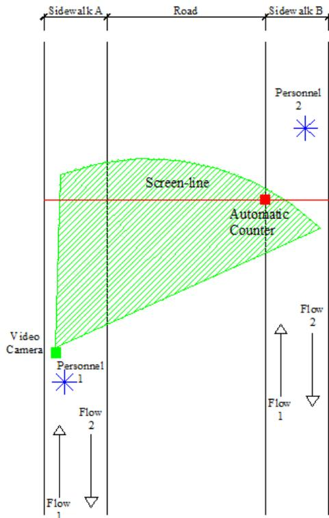
Figure 12. Elements of a counting section.
