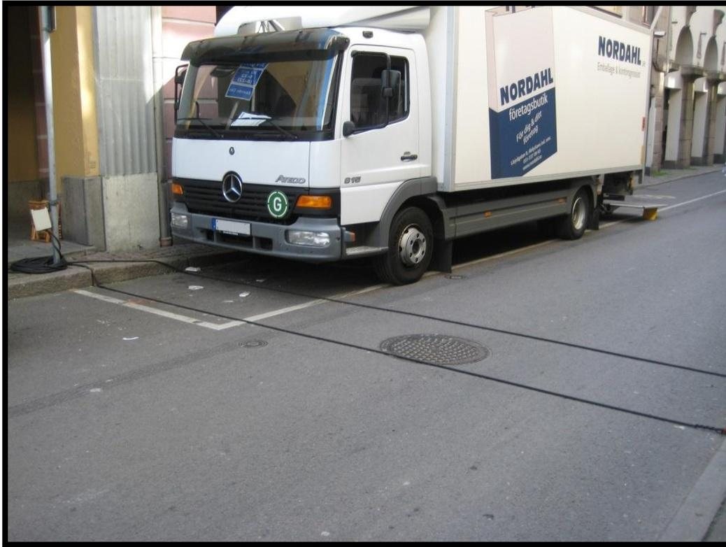
Figure 17. Pneumatic tubes sensors for counting vehicles in Drottninggatan; black tubes on the street.
