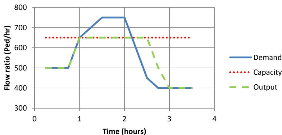
Figure 2. Demand versus Capacity for pedestrian traffic (modified from Roess, et al., 2004). The output reflects how the demand is delayed in time, increasing the usage time.
