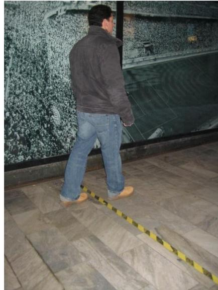
Figure 13. A yellow tape adhered to the pavement was used as the indicator for the imaginary line in the screen-line counting method.
