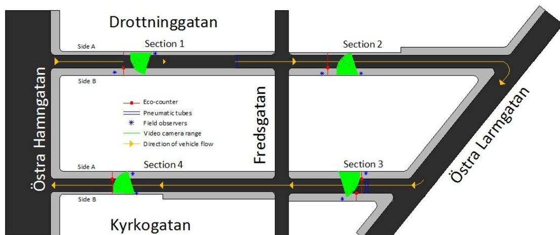
Figure 9. Location of automatic counters, pneumatic tubes, personnel counting and coverage range of the video camera for each section.
