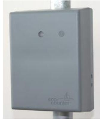
Figure 16. Automatic counter used, Eco-counter passive infrared dual-sensor (Eco-counter, 2010)
