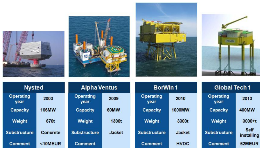
Figure 32 Development in offshore substations
