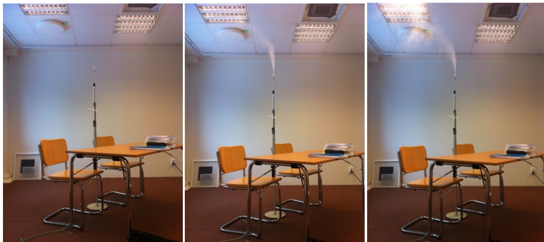
Figure 3.6 (left). A smoke test was performed to illustrate the airflow pattern. The picture shows the smoke gas tests settings just before activating the smoke generator.
