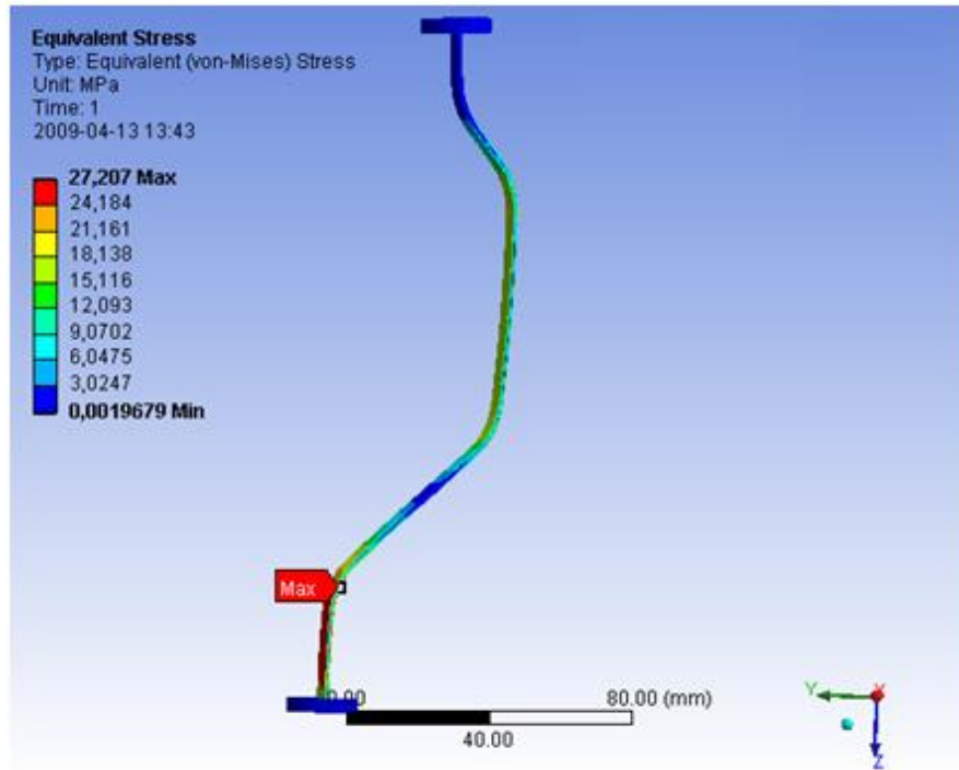
Figure 71. The equivalent stress (von-Mises) for the waveguides.
