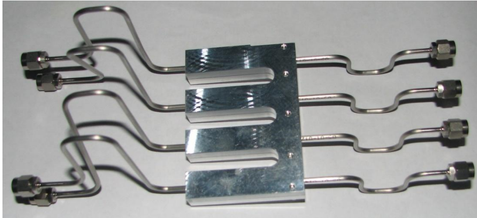
Figure 32. IF cable assembly with 110K thermal shield installed; the two stress-relief half-loops are made for the cable length between the base plate and the 110 K plate and the 110 K and 15 K plates.
