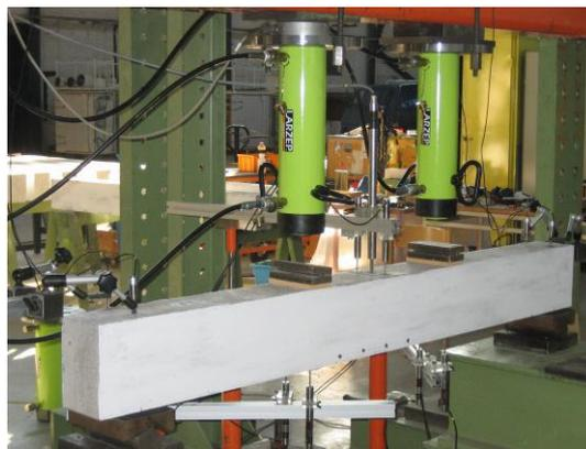
Figure 5.9 Set-up for the beam-bending tests, from Gustavsson and Karlsson (2006).
