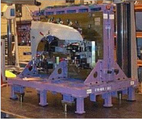
FIGURE 3: POSITIONING OF A FRONT FENDER IN AN INSPECTION FIXTURE.
