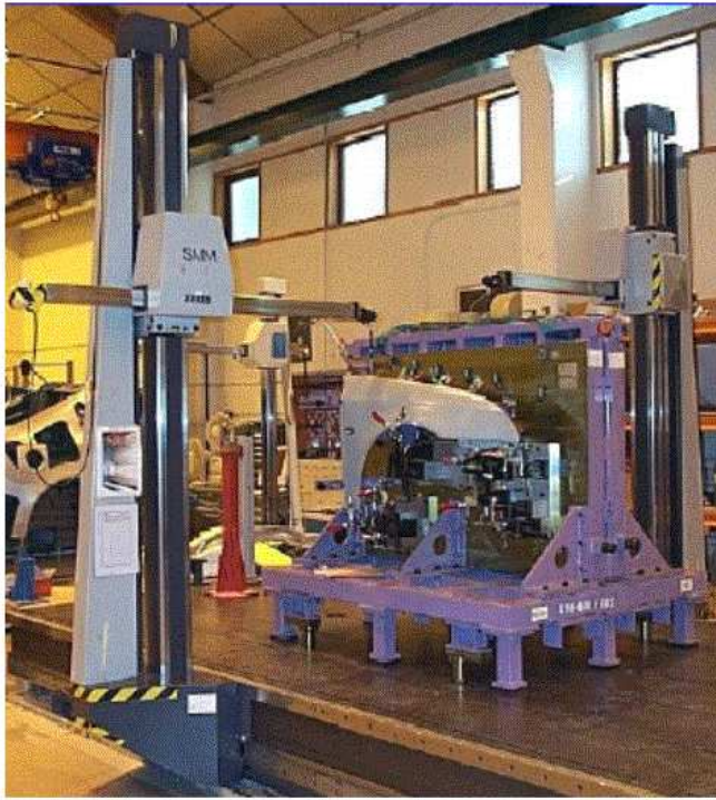
Figure 1.6: A front fender is measured in a CMM.
