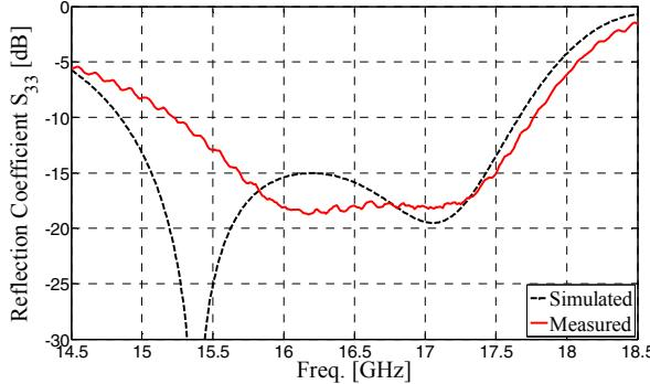
Fig. 7 Simulated and Measured reflection coefficient of port 3
