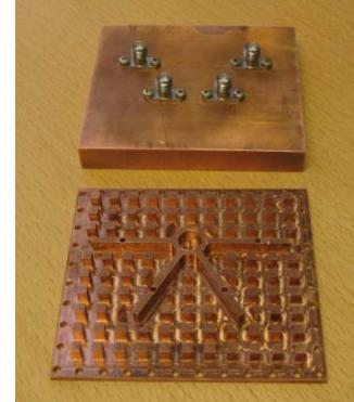
Fig. 1. Photo of the 15 – 17.5 GHz 3dB hybrid in ridge gape waveguide. The texture plate showing the ring hybrid surrounded by metal pins.
