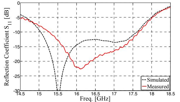
Fig. 3 Simulated and measured reflection coefficient  $S_{11}$
