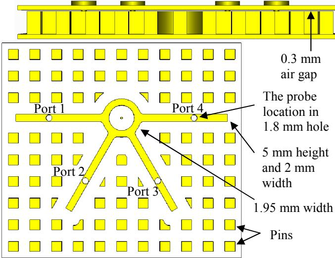
Fig. 2. Geometry of the Ridge gap waveguide hybrid.
