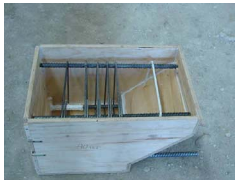
Figure 3.3. Photo of a fabricated mould for a beam-end specimen.
