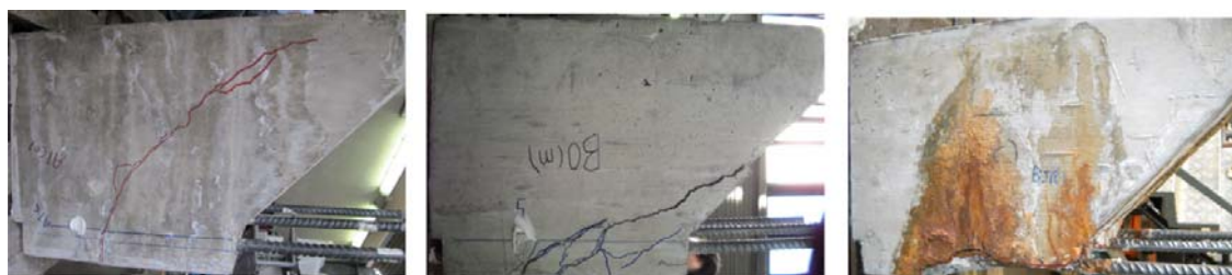
Failure of the test specimen (F)
