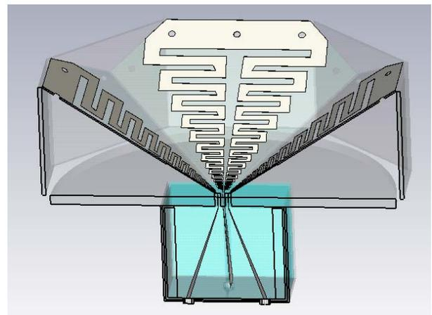
Figure 7. Integration of the balun with Eleven feed petals.
