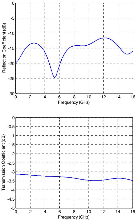
Figure 5. Computed S-parameters of the  $200 \Omega$  4-port solution with  $200 \text{ ohm}$  loads on the 4 differential ports.
