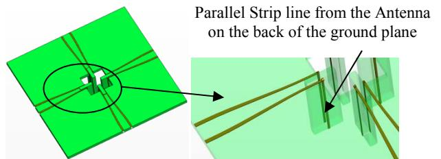
Figure 4. New design of 200 ohm 4-port solution.
