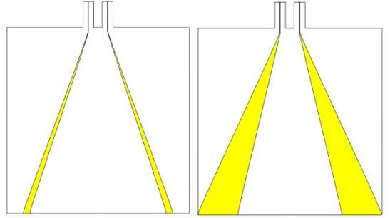
Figure 6. Geometry of the present twin tapered microstrip line balun shows the front (left) and rear (right) sides of the circuit board
