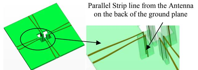
Figure 4. New design of 200 ohm 4-port solution.
