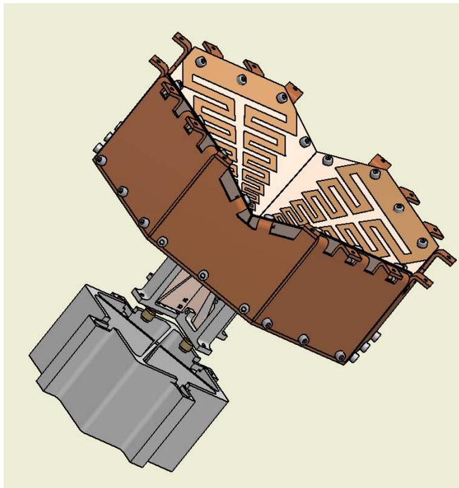
Figure 8. Arrangement of four baluns behind the ground plane for two polarization of Eleven Antenna.
