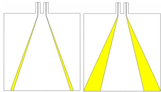
Figure 6. Geometry of the present twin tapered microstrip line balun shows the front (left) and rear (right) sides of the circuit board
