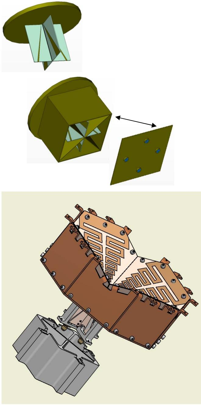
Figure 8. Arrangment of four baluns behind the ground plane for two polarization of Eleven Antenna.
