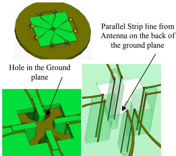
Figure 2. New design of the single ended 8-port solution.
