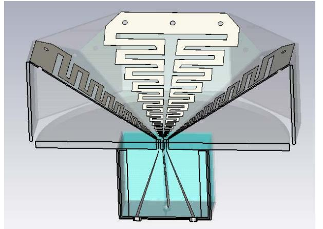
Figure 7. Integration of the balun with Eleven feed petals.
