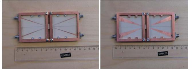
Figure 9. Tapered microstrip balun with back – to – back configuration.
