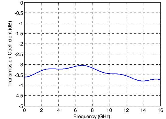
Figure 3. Simulated S-parameters of the single ended 8-port solution.
