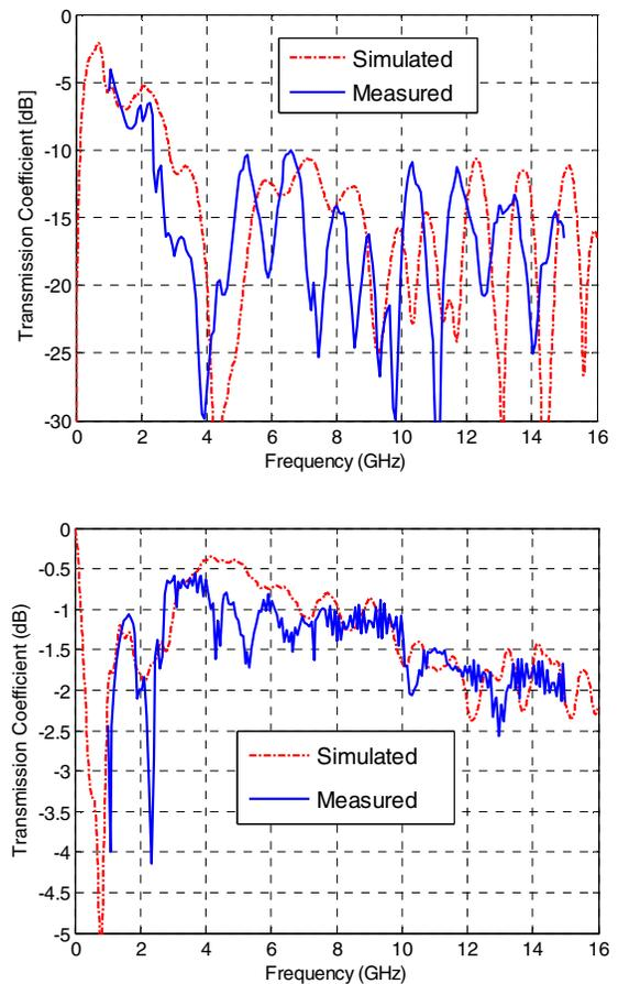
Figure 10. Simulated and Measured S-parameters of back-to-back balun.
