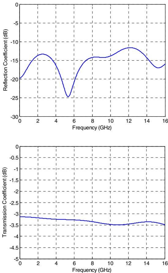
Figure 5. Computed S-parameters of the 200 Ω 4-port solution with 200 ohm loads on the 4 differential ports.
