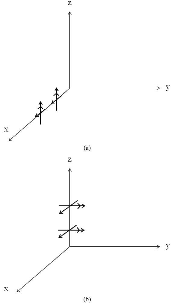
Fig. 1 Huygen's source pair: (a) parallel-collinear arrangement; (b) double parallel arrangement
