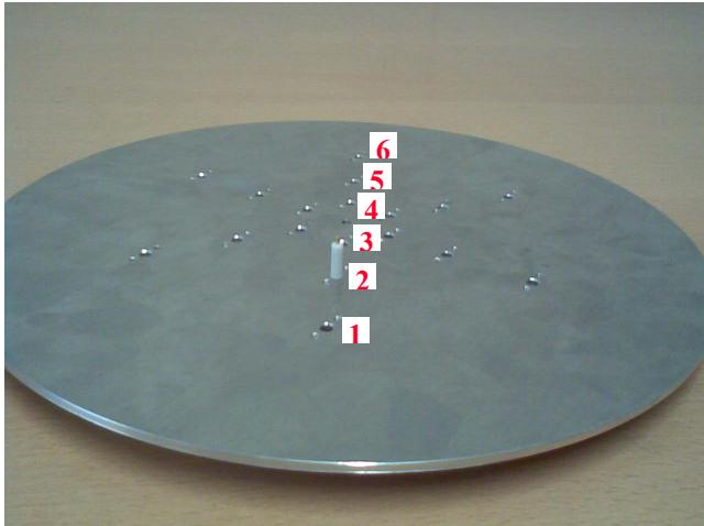
Fig. 5 Photo of monopole mounted on the ground plane.
