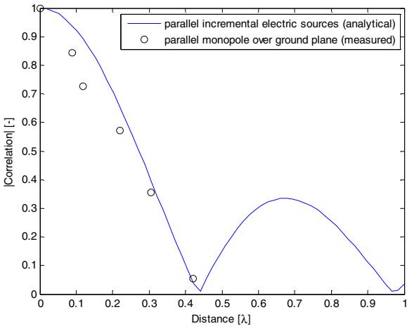
Fig. 6 Measured spatial correlation of parallel monopole in reverberation chamber against that of theoretical parallel incremental electric source.
