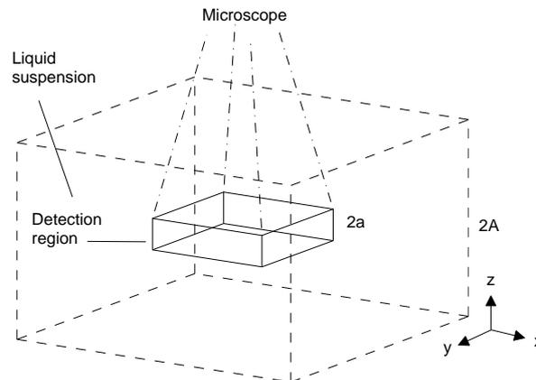
Figure 2.1: An illustration of the experimental setup. The detection region is modeled as a rectangular box centered in the liquid suspension. Particles outside the detection region cannot be observed. The tracking depth is  $2a$ , and the thickness of the liquid suspension is  $2A$ .
