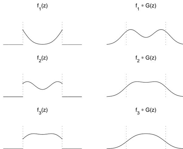
Figure 2.3: Illustration of the procedure for computing the track length distribution.  $f_1(z)$  is the probability density of a particle that has just entered the detection region according to Eq. (2.2). Truncation outside of  $[-a, a]$  of the convolution  $f_1 * G(z)$  yields a non-normalized density  $f_2(z)$  which integrates to the probability that the particle still remains in the detection region for a second sampling time point, and so forth.
