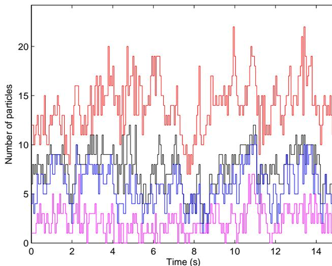
Figure 2.6: Experimentally observed process values for minimum contrast thresholds  $C_{\text{min}} = 1.2$  (red),  $C_{\text{min}} = 1.4$  (black),  $C_{\text{min}} = 1.6$  (blue), and  $C_{\text{min}} = 1.8$  (magenta). Naturally, the process values are monotonically decreasing with increasing threshold.
