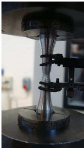
Figure 6. Necking of a ductile and heterogeneous material
